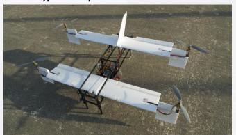
Ardupilot Mega (microprocessor and sensor) is used to stabilize the UAV during hovering and forward flight using its 3-axis gyroscope and accelerometer.
