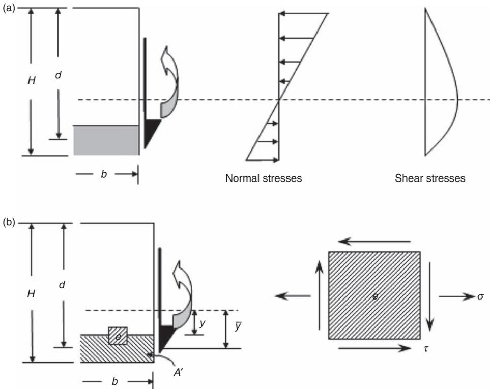
**Figure 10.** (a) Normal and shear stresses distribution, (b) element extracted from section subjected to normal and shear stresses.
