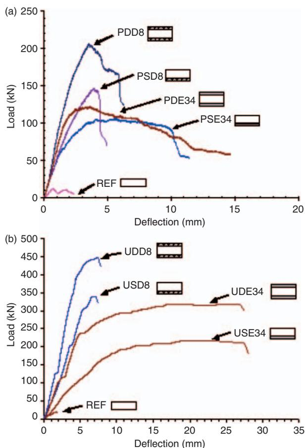
Figure 6. Load deflection responses of: (a) Series I test walls (b) Series II test walls.
