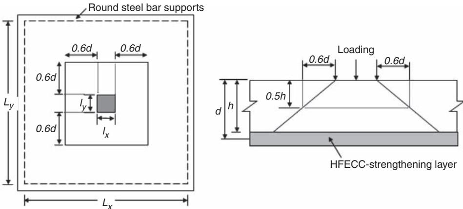
Figure 9. Observed critical punching shear perimeter.
