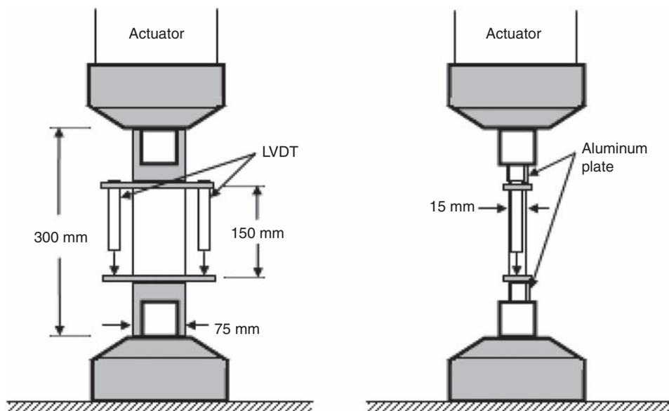
**Figure 2. Plan view and side view of tensile coupon test.**
