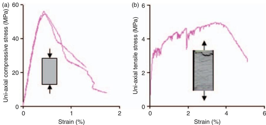
**Figure 1.** Typical stress–strain curves of HFECC: (a) uni-axial compression and (b) uni-axial tension.
