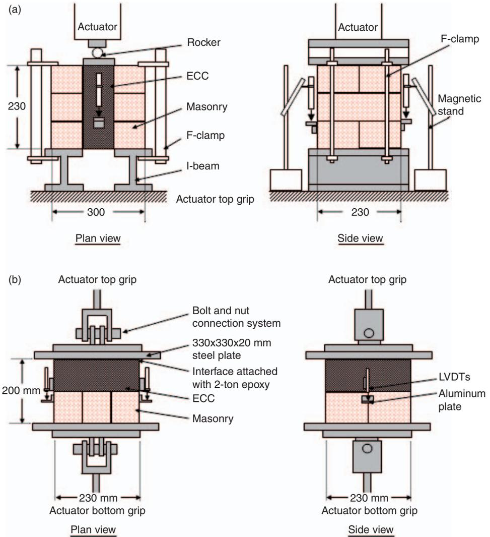
**Figure 4.** (a) Plan view and side view of direct shear test, (b) plan view and side view of uni-axial tensile-bond test.
