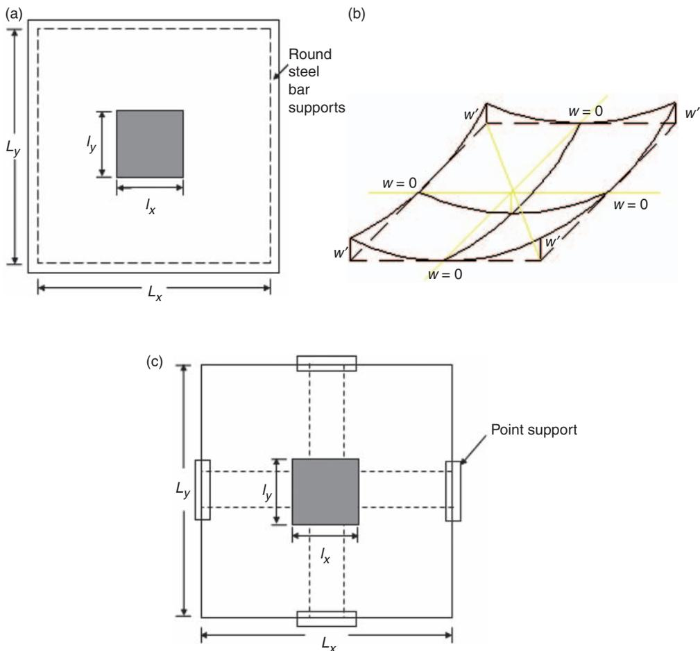
**Figure 11.** (a) Plan view of experimental set-up, (b) uplifting at the corners, (c) panel resting on four-point supports.
