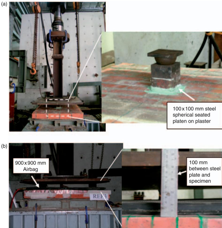
**Figure 5.** (a) Series I – patch loading test set-up, (b) Series II – uniformly distributed loading test set-up.
