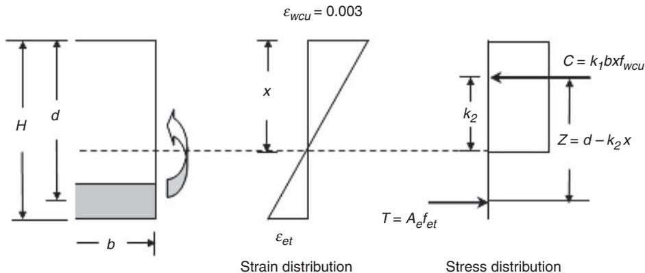
**Figure 8.** Section analysis for flexural failure.
