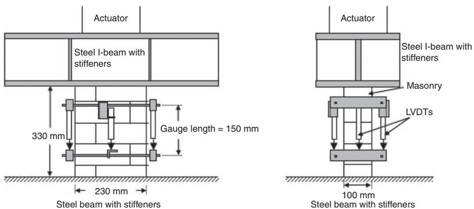
Figure 3. Plan view and side view of masonry wallette compression test.
