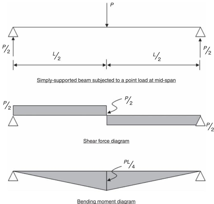
Figure A1. Simply supported beam subjected to point load.
