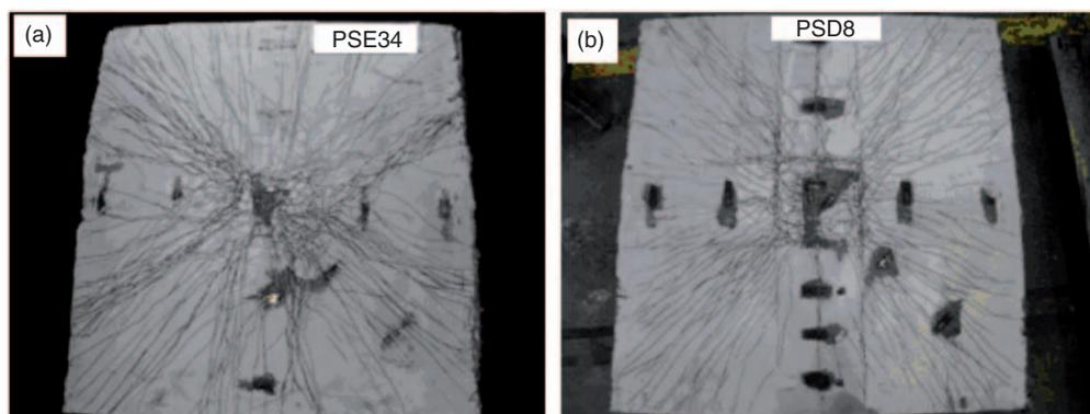
Figure 7. Typical cracking pattern of HFECC-strengthening layer: (a) without steel mesh (b) with steel mesh.
