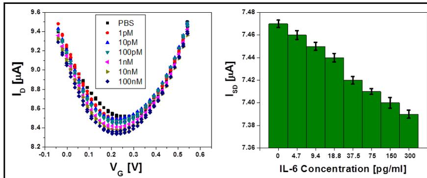
Figure 4. (a) Drain current vs. gate voltage curve obtained with different concentration of IL-6 concentrations. (b)  $I_{SD}$  characteristic measurement with different clinically relevant concentrations of IL-6 protein at fixed gate voltage.
