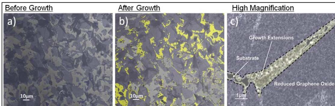
Figure 1. SEM images of (a) GO flakes before ethanol CVD treatment with ca. 60% coverage (b) reduced GO flakes after 30-minutes CVD treatment with ca. 75% coverage in total. (c) high-magnification on the new growths between two reduced GO flakes. [GO flakes and new carbon growths are highlighted in purple and yellow respectively]
