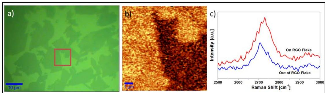
Figure 2. (a) Optical microscope image of 2-hour processed reduced GO flakes on  $SiO_2$  substrate (b) Raman mapping at edges of RGO flakes showing 100% carbon coverage. (c) Raman spectrum of both on and out of RGO flakes.
