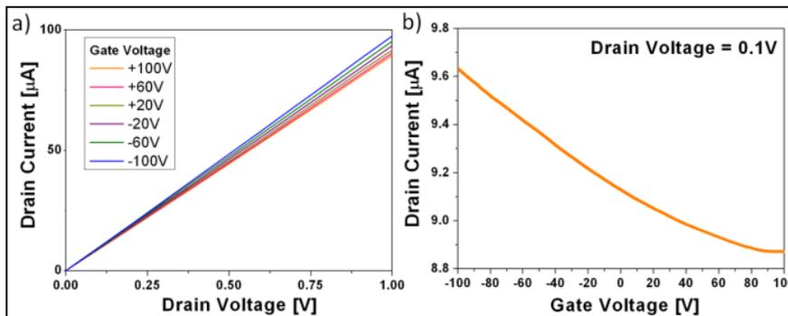
Figure 3. (a)  $I_d$ – $V_d$  output characteristics under different applied  $V_g$  (b)  $I_d$ – $V_g$  transfer curve of the ethanol CVD-processed reduced GO transistor device.
