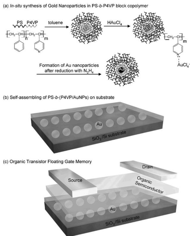
**Fig. 1** Schematic illustration of (a) micellation process with *in-situ* synthesis of Au nanoparticles in PS-*b*-P4VP block copolymer; PS-*b*-(P4VP/AuNPs), (b) the self-assembly of PS-*b*-(P4VP/AuNPs) micellar film on substrate and (c) cross-section of an organic field-effect transistor (OFET) using PS-*b*-(P4VP/AuNPs) as floating gate memory elements.
