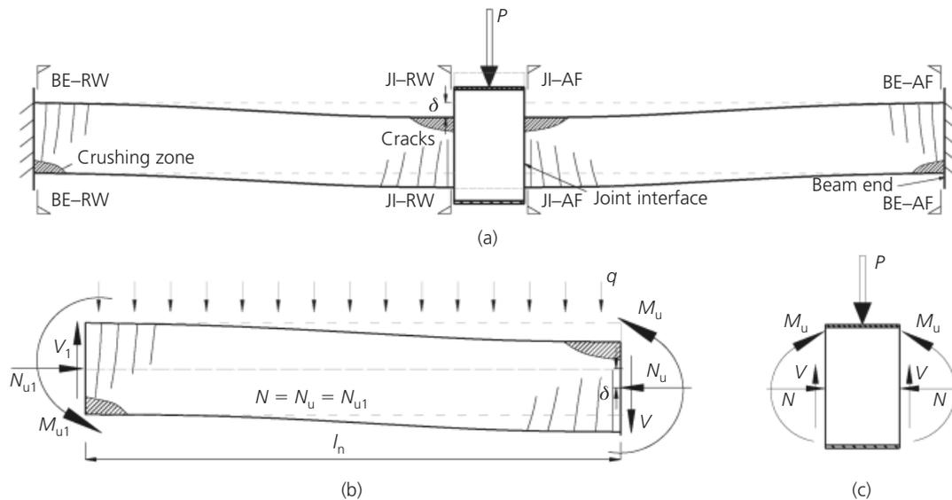
**Figure 1.** Free body diagrams of RC sub-assemblage at CAA:
