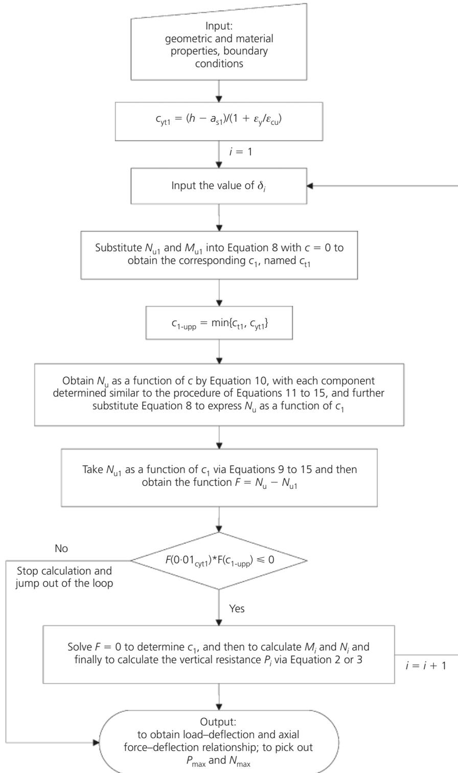
Figure 6. Procedure for calculation of vertical resistance and internal force
