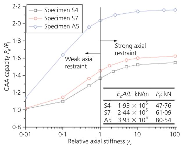
Figure 10. Effect of axial restraint stiffness on CAA capacity
