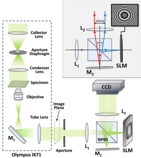
Fig. 1. Experimental setup; NPBS, nonpolarizing beam splitter;  $M_1$ ,  $M_2$ , mirrors;  $L_1$ ,  $L_2$ , lenses; SLM, spatial light modulator. The inset shows one light path along the optical axis with zero local tilt.
