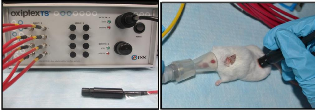
Figure 1. Photograph of the front panel of the DOS control module (left) and the use of a contact probe on a mouse model under inhalable anesthesia (right).
