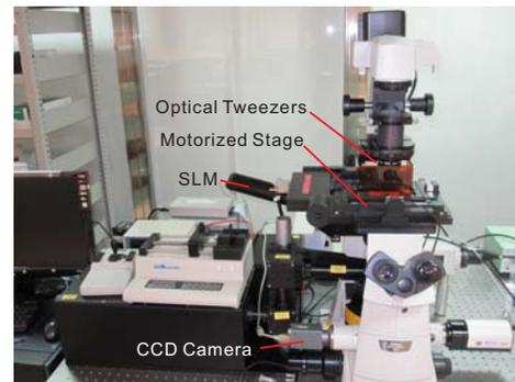
Fig. 7. A robot-tweezer manipulation system.
