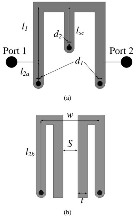
Figure 2. Proposed second-order filter configurations: (a) Layer 1 and (b) Layer 3.
