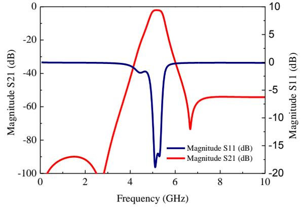
Figure 5. Simulation results of proposed fourth-order filter.
