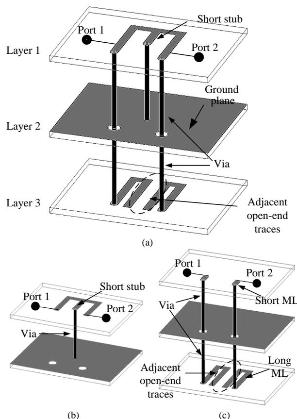
Figure 1. Proposed second-order filter configuration and equivalent circuits: (a) proposed filter, (b) M-path, and (c) E-path.
