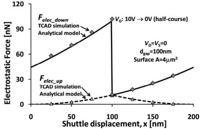
Figure 6. Analytical modeling of electrostatic forces  $F_{\text{down}}$  (shuttle  $\rightarrow$  gate) and  $F_{\text{up}}$  (shuttle  $\rightarrow$  drain/source) vs. shuttle displacement.  $V_G$ -pulse turn-off is applied after shuttle  $\frac{1}{2}$ -course. Solid markers represent TCAD solutions (Coventorware simulations).
