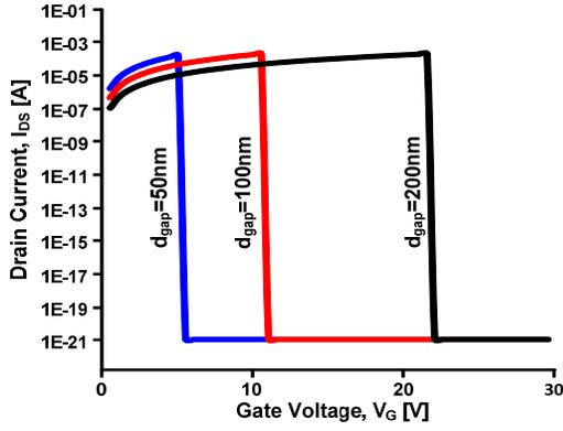
Figure 8. Plot of  $I_{DS}$  vs  $V_G$  of the shuttle based NEM memory cell for different actuation gap thickness ( $V_{DS} = 0.2V$ ).
