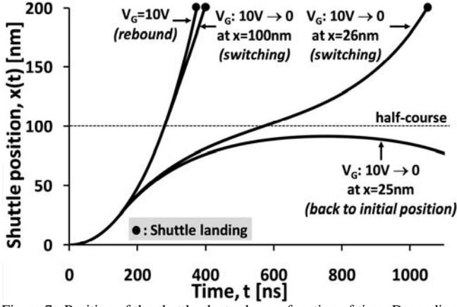
Figure 7. Position of the shuttle electrode as a function of time. Depending on the duration of the  $V_G$  pulse, three cases could happen: (i) the shuttle back to its initial position if pulse duration is too short, (ii) proper switching or (iii) shuttle electro-mechanical rebound if the pulse is too long.
