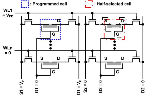
Figure 11. Proposed memory array structure using NEM memory device and two MOS transistors (1NEM-2T).
