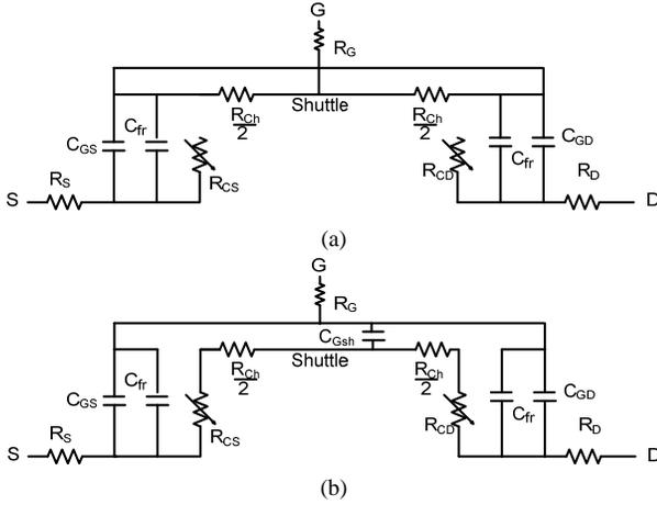
Figure 3. Electrical equivalent circuits: (a) down-state, (b) up-state.
