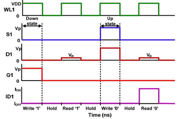
Figure 12. NEMs NVM cell read and write operations.
