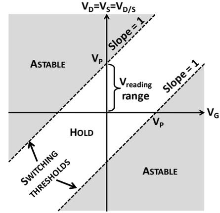
Figure 4. Stability and switching thresholds of the NVM device.
