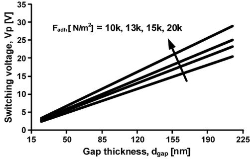
Figure 10. Plot of gate switching voltage as a function of gap thickness for different adhesive forces.
