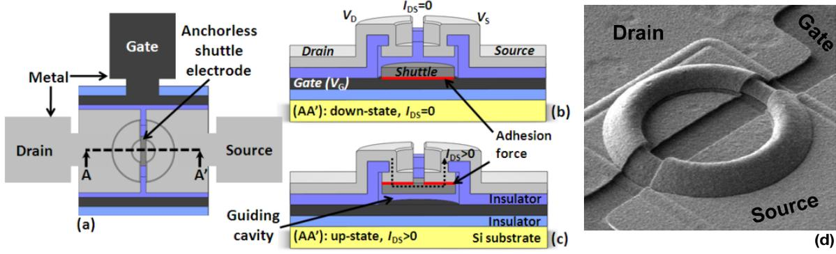
Figure 2. Proposed 3-terminal shuttle NEM memory device: (a) top-view layout, (b) AA' 3D cross section in the down-state, (c) AA' 3D cross section in the up-state. (d) Experimental circular test structure. Two metal electrodes (source and drain) are visible. A circular guiding pod is defined all around the circular shuttle to provide lateral guiding of the free shuttle.
