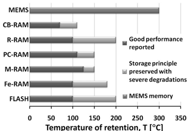
Figure 1. Maximum temperature of operation for various types of non-volatile memories. This review is based on recently published papers, constrains are more stringent for commercial memories [7]-[17].
