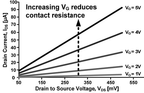
Figure 9. Plot of drain current ( $I_{DS}$ ) of the shuttle based NEMs device as a function of  $V_{DS}$  for different  $V_G$ .
