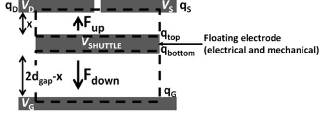
Figure 5. Double air gap capacitor divider with charge distribution. While switching, the shuttle electrode carries a fixed charge.
