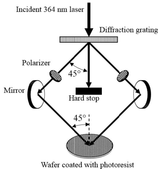
Figure 3. Schematic representation of the experiment setup
