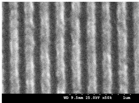
Figure 4. SEM image of line features patterned using single exposure with the two-beam IL system
