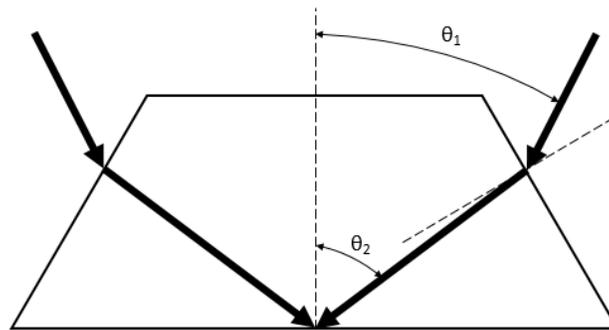
Figure 2. Schematic representation of beams refracted from  $\theta_1$  to  $\theta_2$  and finally interfering at the bottom surface of the prism
