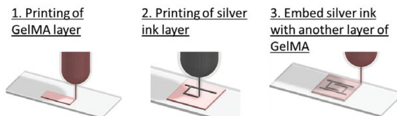
Figure 1. Schematic of the bioprinting process using microvalve for fabricating the bioelectronics platform with electronic circuit sandwiched between hydrogel layers.
