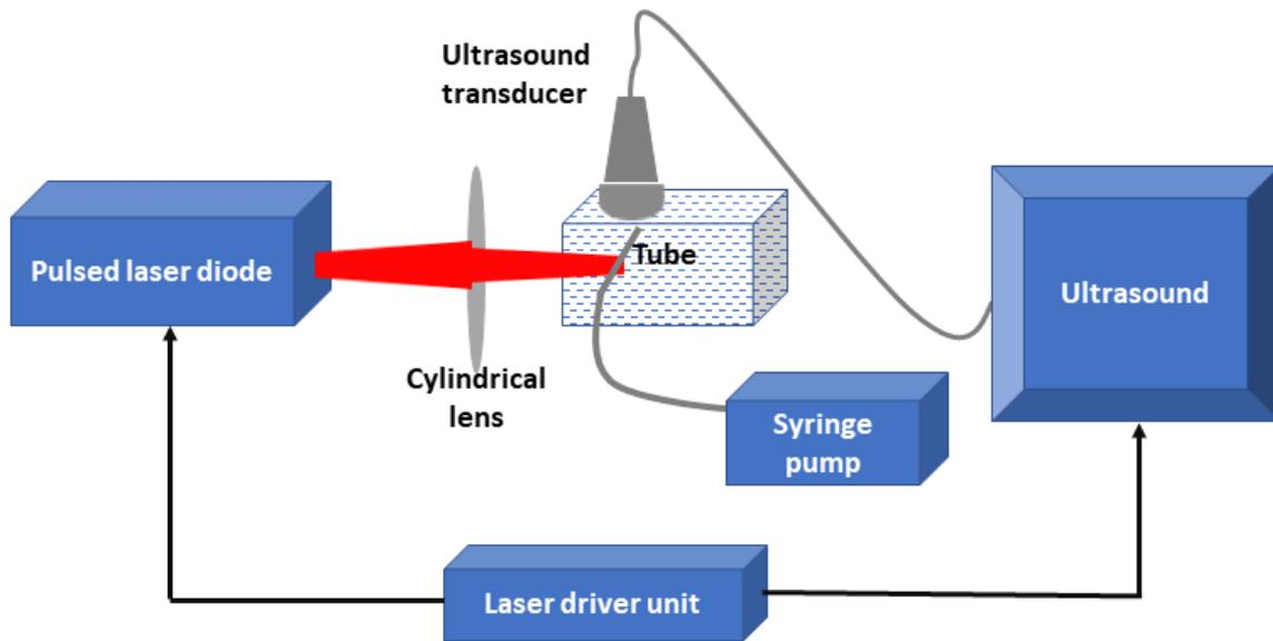
Figure 1: Schematic representation of the high framerate PLD-PAT imaging system
