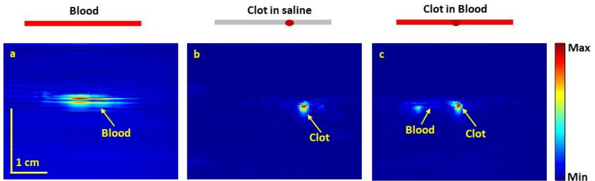
Figure 2: (a) PA image of blood in LDPE tube, (b) PA image of clot in saline, (c) PA image of clot in blood. Scale bar and color bar are mentioned in the image.
