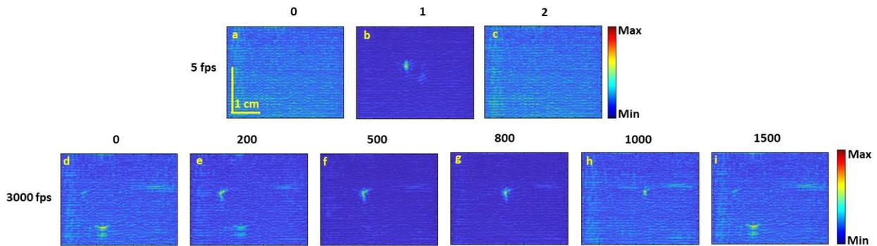
Figure 3: (a-c) PA images of the clot in blood flowing at a velocity of 5 cm/s imaged at a framerate of 5 fps; (d-i) PA images of the clot in blood flowing at a velocity of 5 cm/s imaged at a framerate of 3000 fps. Scale bar, color bar and frame number are mentioned in the images.
