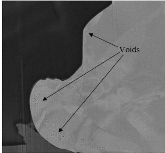
Fig.12 Nano voids formed in the PdCu wire bond in the as-bonded state
