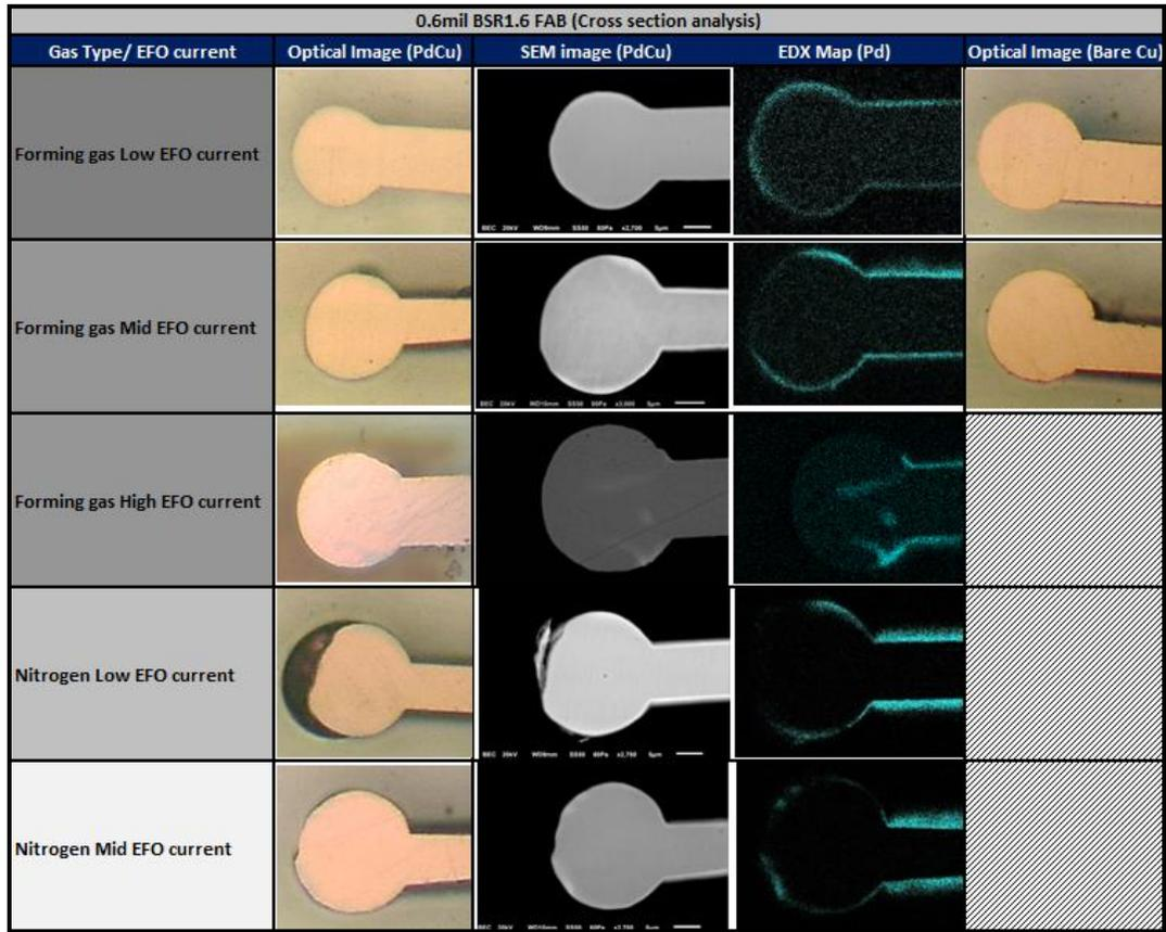
Fig. 2 FAB cross-sections for PdCu and bare Cu wires
