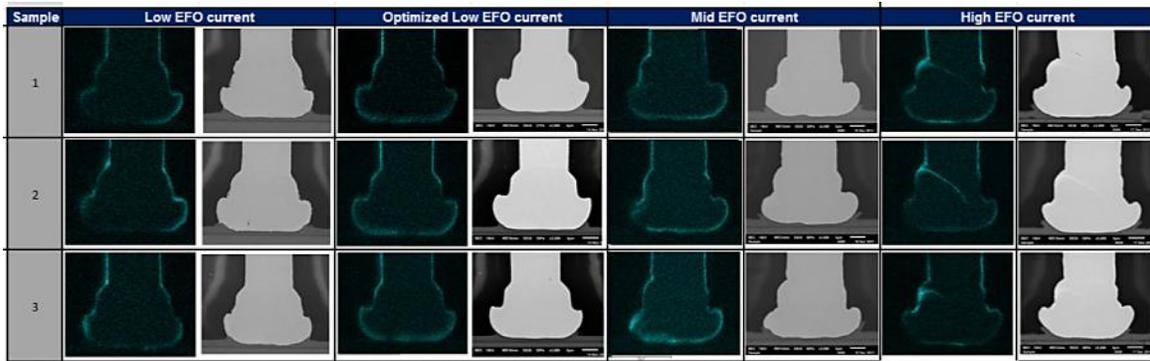
Fig. 10 EDX elemental map showing Pd distribution for bonded ball at various EFO current settings
