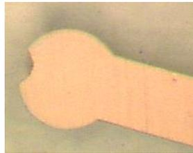
Fig.3 Example of an apple bite FAB observed at low EFO current in forming gas
