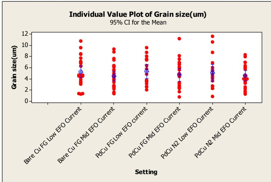
Fig. 7a Individual value plot of FAB grain size at different settings
