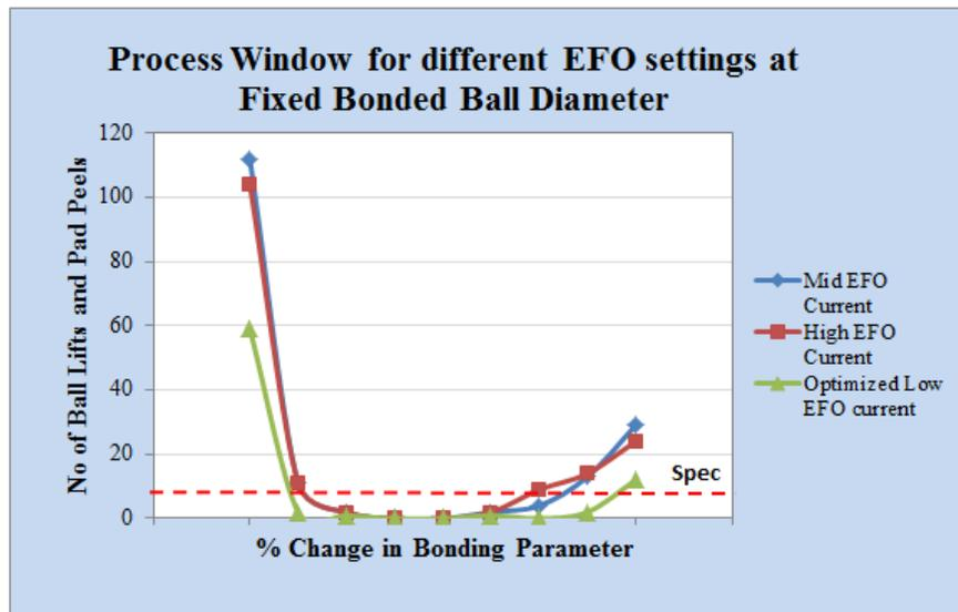
Fig. 11 Process window for different EFO current setting in forming gas
