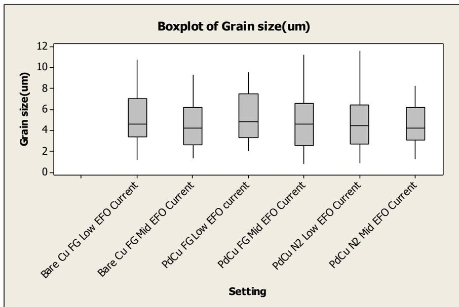
Fig. 7b Box plot of FAB grain size at different settings
