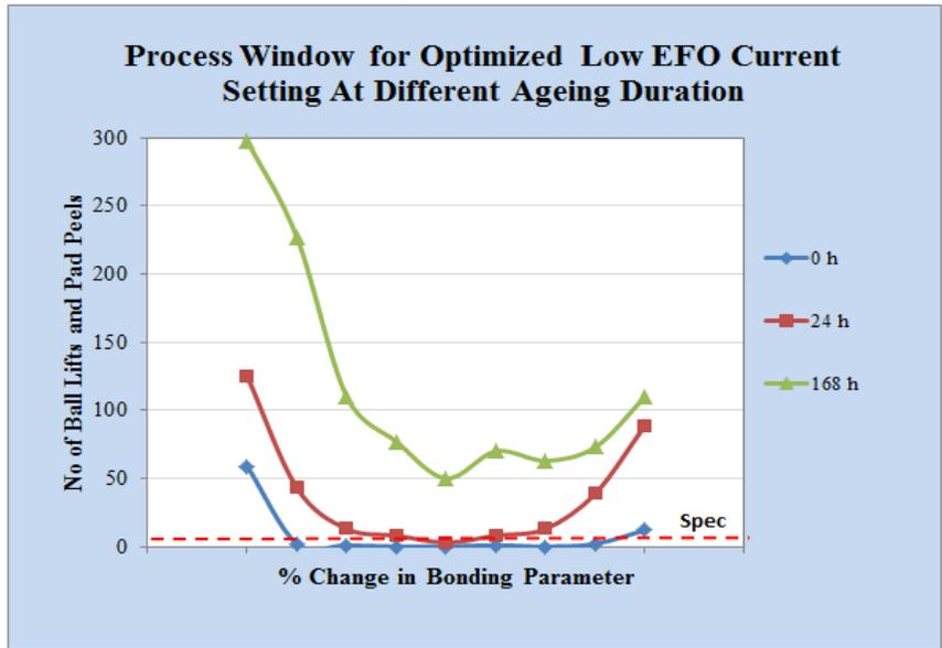
Fig. 15 Process window for optimized low EFO current setting at different annealing durations
