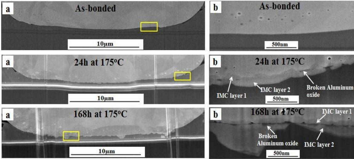
Fig. 14 Comparison of IMC growth along a) Entire bond interface with yellow box showing the zoomed in sections and at b) Zoomed in sections
