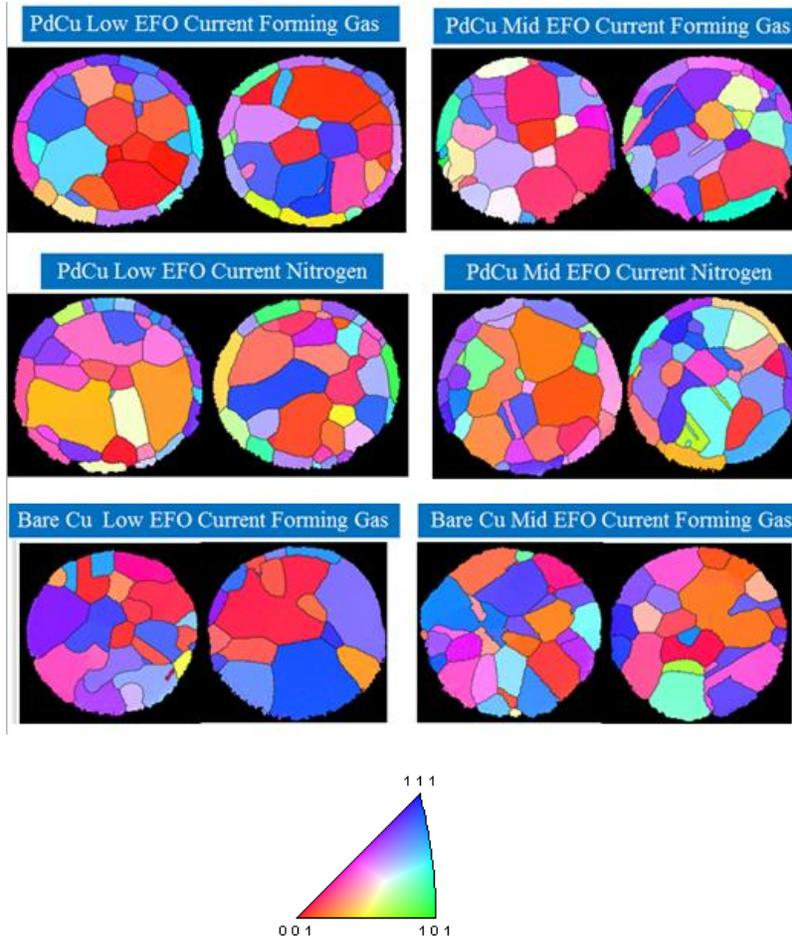
Fig.6 EBSD images of PdCu and bare Cu wire across the FAB
