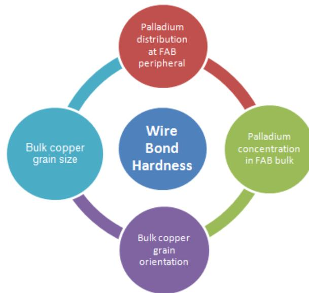
Fig. 9 Impact diagram showing factors affecting FAB hardness
