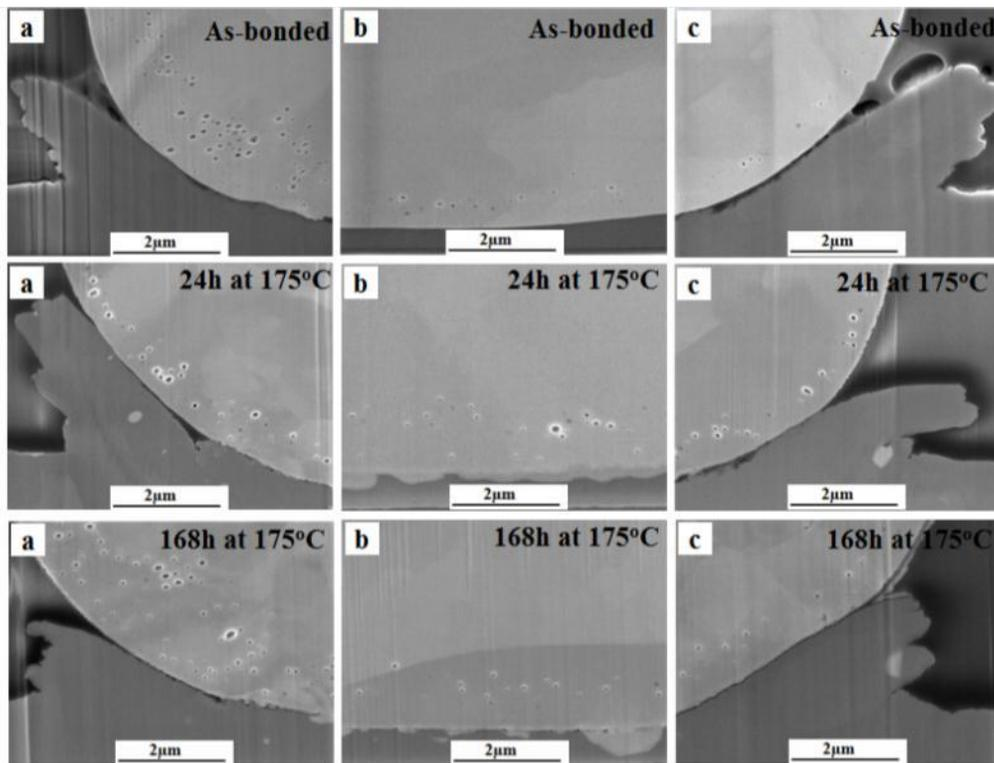
Fig. 13 Voids in a) Left periphery, b) Centre, c) Right periphery of bond interface at different annealing time
