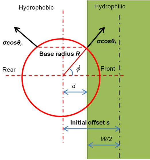
Fig. 5 Plan view of droplet which straddles across sharp wettability contrast
