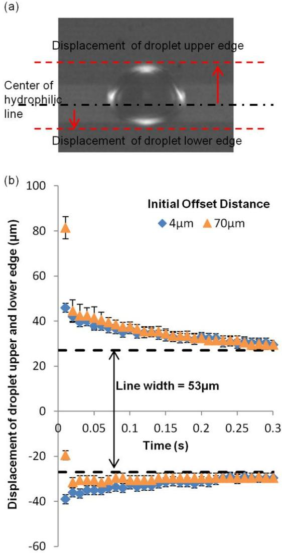
Fig. 4 (a) Definition for displacement of upper and lower edges of droplet relative to center of hydrophilic strip. (b) Time evolution of upper and lower edges of droplet relative to hydrophilic line.
