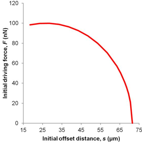
Fig. 6 Theoretical driving force on droplet induced by wettability contrast at various offset distances. Hydrophilic line width  $W = 53\mu\text{m}$ . Droplet base radius  $R = 45\mu\text{m}$
