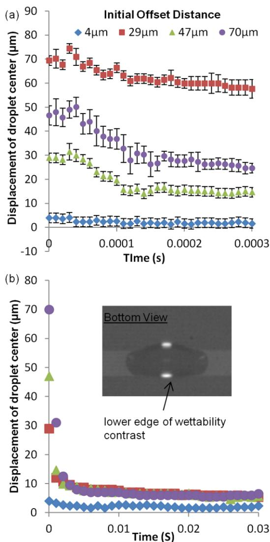
Fig. 3. Displacement of droplet center from center of hydrophilic line at different initial offset distances (a) for short time scale (b) for longer time scale. Inset shows that the lower edge of the wettability contrast impeded the completeness of centering process. Error bar is not shown in (b) for clarity.
