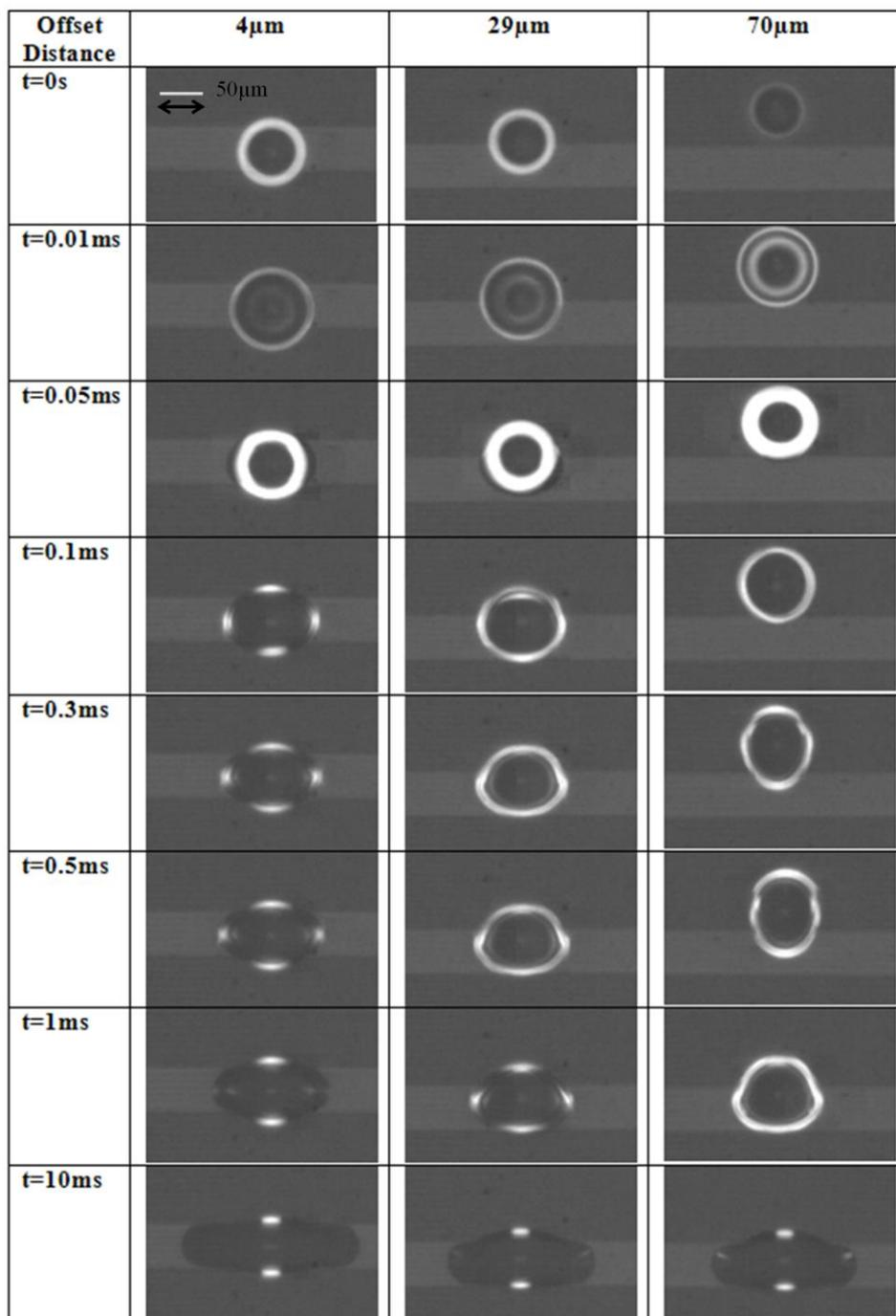
Fig. 2. Bottom view of droplet impingement and spreading on hydrophilic line on PET surface.
