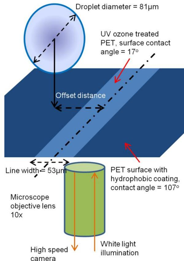
Fig. 1. Experimental setup for high speed imaging of micro-sized droplet impinging and spreading on hydrophilic line.
