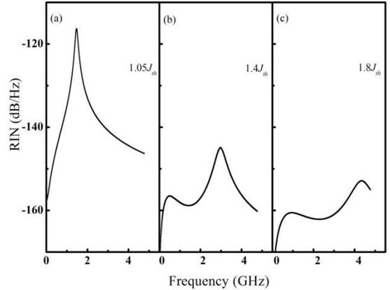
Fig. 3. The RIN spectra for hybrid laser with a 3  $\mu\text{m}$  III-V ridge width, 220 nm Si ridge height under different injection current density: (a) Injection current density is 1.05J<sub>th</sub>; (b) Injection current density is 1.4J<sub>th</sub>; (c) Injection current density is 1.8J<sub>th</sub>.
