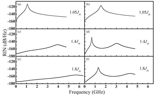
Fig. 6. Comparison of the RIN spectra for a hybrid laser (a) (c) (e) and diode laser (b) (d) (f) with same ridge width of  $4\mu\text{m}$ , under different injection current densities: Injection current density is  $1.05J_{th}$  (first row); Injection current density is  $1.4J_{th}$  (second row); Injection current density is  $1.8J_{th}$  (third row).
