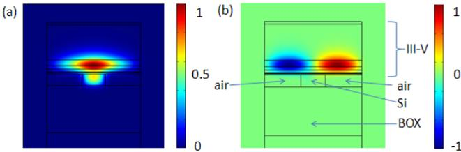
Fig. 1. The optical field distributions of the  $\text{TE}_{00}$  (a) and  $\text{TE}_{10}$  (b) mode of a hybrid laser with a 4 $\mu\text{m}$ -wide III-V ridge, a 1 $\mu\text{m}$ -wide and 500 nm-high Si ridge with arrows indicating the silicon-on-insulator (SOI) structure. BOX in (b) refers to buried oxide.
