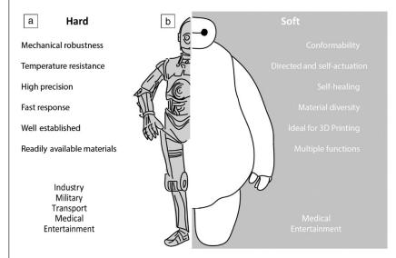
**Figure 2.** Selected properties and applications of traditional hard robots versus soft robots. The cartoons represent (a) a famous metallic humanoid<sup>4</sup> and (b) a soft character.<sup>11</sup>
