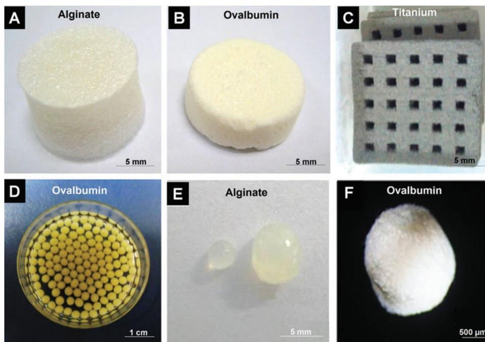
**FIG. 1.** Images of three-dimensional (3D) (A–C) scaffolds, (D, E) hydrogels, and (F) microcarriers of various geometry, size and morphology used in tissue engineering applications. Color images available online at [www.liebertpub.com/teb](http://www.liebertpub.com/teb)
