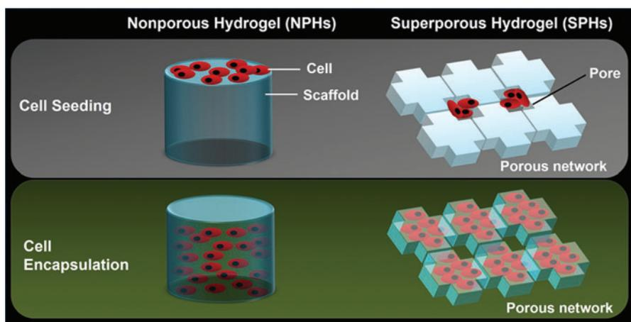
**FIG. 5.** Schematic illustration of cell culture for nonporous hydrogels (NPHs) and superporous hydrogels (SPHs). Cell seeding onto NPHs will result in cells proliferating on the surface, while cell encapsulation entraps cells within the scaffold. For SPHs, cells will proliferate between the pores when they are seeded onto the scaffolds, or entrapped in the interior during the encapsulation process. Color images available online at [www.liebertpub.com/teb](http://www.liebertpub.com/teb)
