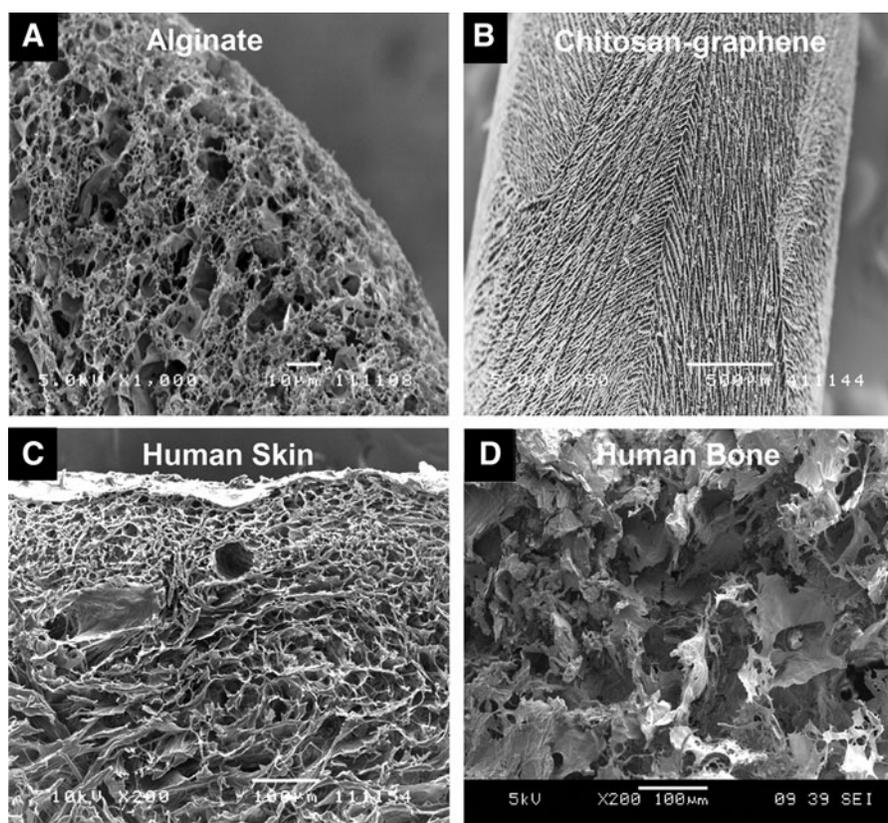
**FIG. 2.** Scanning electron microscopy (SEM) images of (A, B) porous scaffolds and (C, D) human tissues with interconnected pores. Tissue engineered scaffolds should ideally mimic the porosity, pore size, and function of native human tissues.
