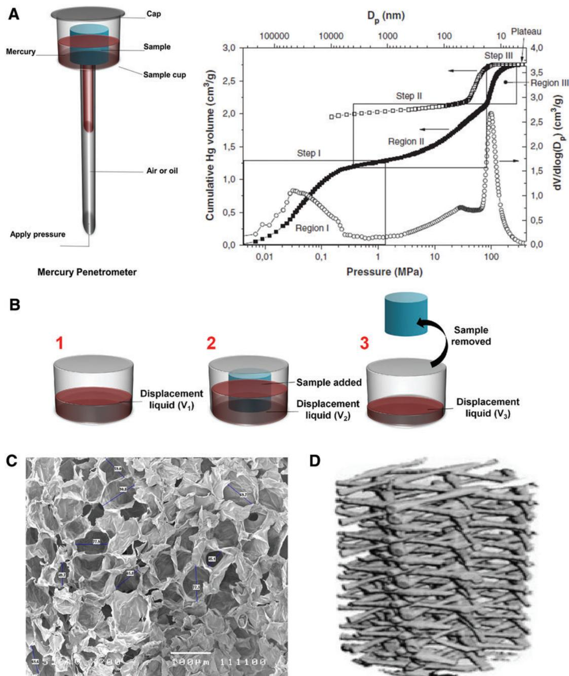
**FIG. 6.** Schematic illustration of (A) mercury porosimetry, (B) three-step liquid displacement process, (C) SEM imaging technique, and (D) microcomputed tomography imaging used for porosity or pore size measurement of scaffolds. Images adapted and reproduced by permission of Elsevier and IOP Publishing Ltd. (DOI: 10.1088/1758-5082/3/3/034114).<sup>121,122</sup> Color images available online at [www.liebertpub.com/teb](http://www.liebertpub.com/teb)
