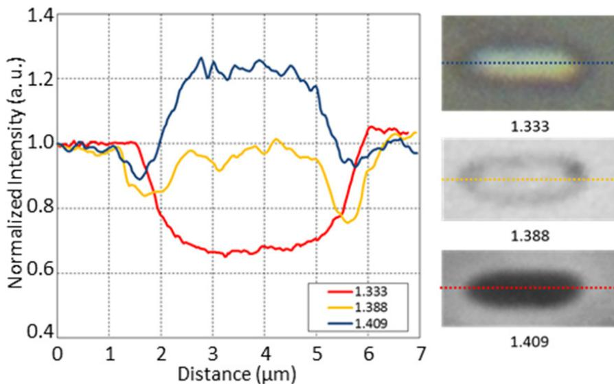
Figure 4: Pixel intensity analysis of an individual *E. coli* cell when the external medium is tuned. The bacteria cell appears to be invisible when the refractive index of the external medium is 1.388.
