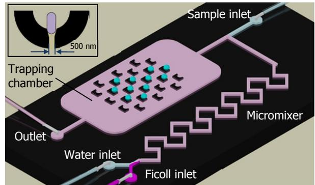
Figure 1: Schematic illustration of the optofluidic chip for biophysical measurement of single bacterium by using null-method in immersion refractometry. Inset shows the trapping structure with a gap of 500 nm.
