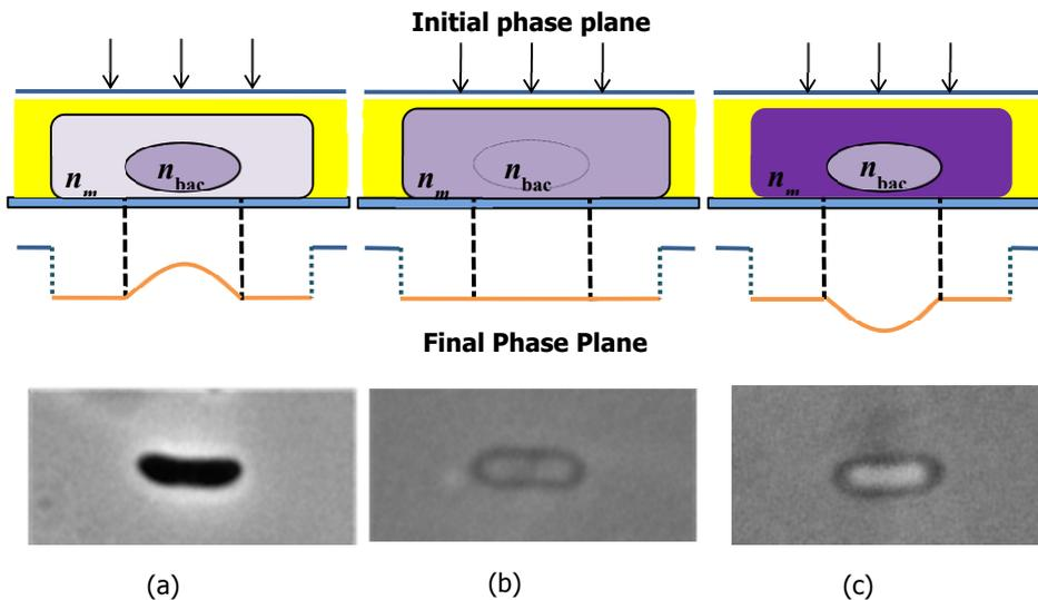
Figure 2: Phase transformation and the phase-contrast microphoto of *E. coli* cell being immersed into a medium with refractive index (a) lower than, (b) same as, and (c) higher than the one of the cell.
