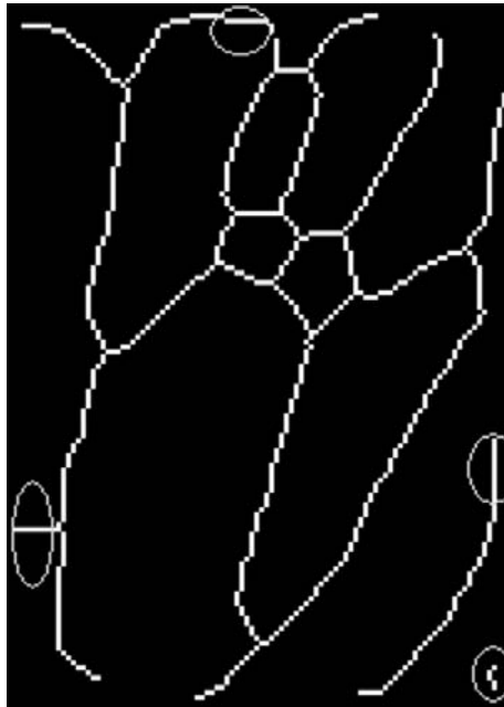
Figure 5.3: Skeletons of the vein pattern using binary-based skeletonization, where the shape of the vein pattern is overall well preserved, but the false branches (in the circled area) are also numerous.
