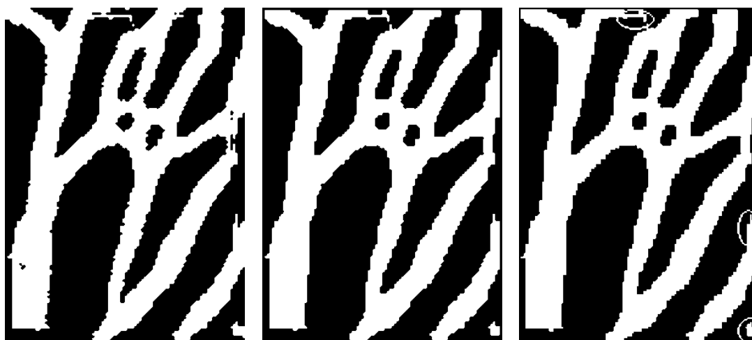
(a) Local Thresholding with Global Reduction for Figure 4.3(a) (b) After Morphological Closing (c) Misclassified background pixels (The circled areas)
