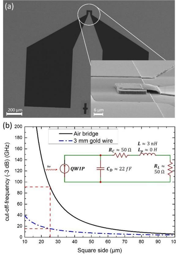
**Fig. 2.** (a) The top view of the QWIP (The inset: zoom-in of the active region with the air bridge); (b) Cut-off frequency at  $-3$  dB as a function of the MESA dimensions for the conventional wire bonding (dashed line) and the proposed air-bridge (solid line) devices (The inset: electrical circuit of the device).
