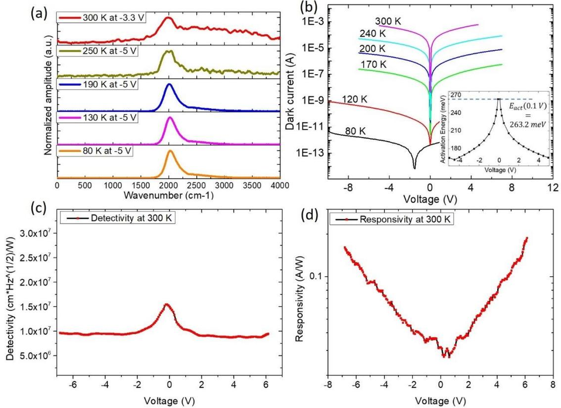
**Fig. 3.** (a) Spectra of the QWIP at several different temperatures up to 300 K; (b) Current-voltage (IV) characteristics in background condition for different temperature, inset: activation energy as a function of the bias voltage; background-limited detectivity (c) and responsivity (d) of the QWIP device at 300 K as a function of the bias voltage.
