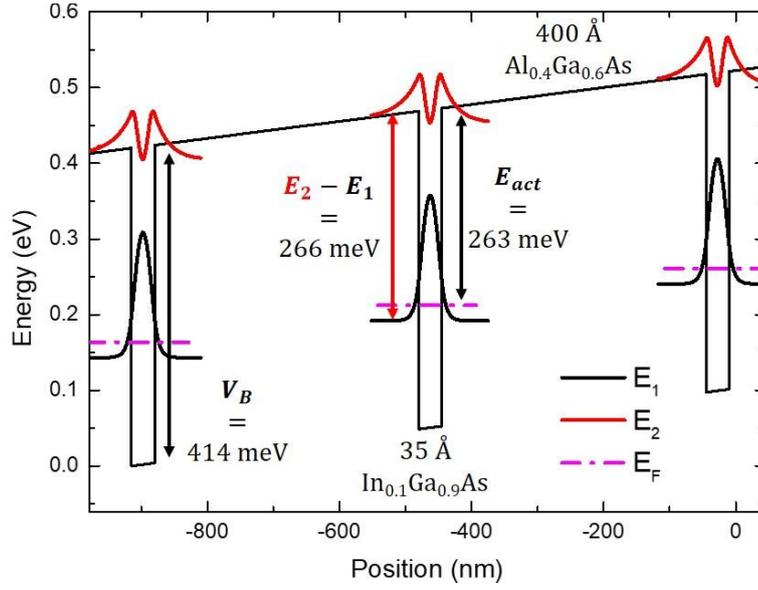
**Fig. 1.** Band-structure of the developed quantum well infrared photodetector (QWIP) with 3 quantum wells (QWs) active regions at a bias voltage of 2 V. The most relevant physical parameters of the structure are indicated in the figure.
