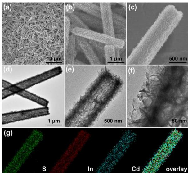
**Figure 3.** (a-c) FESEM and (d-f) TEM images of hierarchical  $\text{In}_2\text{S}_3\text{-CdIn}_2\text{S}_4\text{-10}$  nanotubes, and (g) elemental mappings of a single  $\text{In}_2\text{S}_3\text{-CdIn}_2\text{S}_4\text{-10}$  nanotube.
