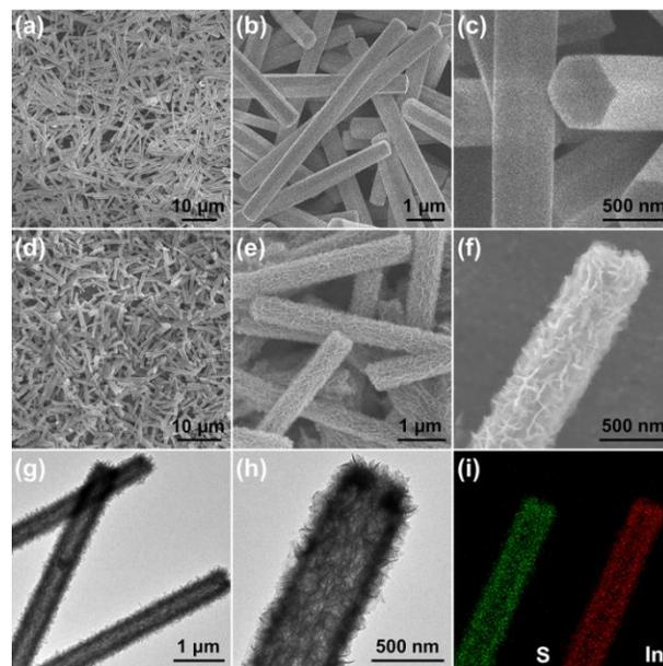
**Figure 2.** (a-c) FESEM images of MIL-68 hexagonal prisms, (d-f) FESEM and (g,h) TEM images of hierarchical  $\text{In}_2\text{S}_3$  nanotubes, and (i) elemental mappings of an individual  $\text{In}_2\text{S}_3$  nanotube.
