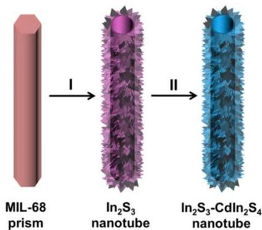
**Figure 1.** Schematic illustration of the synthetic process of the hierarchical  $\text{In}_2\text{S}_3\text{-CdIn}_2\text{S}_4$  heterostructured nanotube. (I) liquid phase sulfidation, (II) cation exchange reaction.
