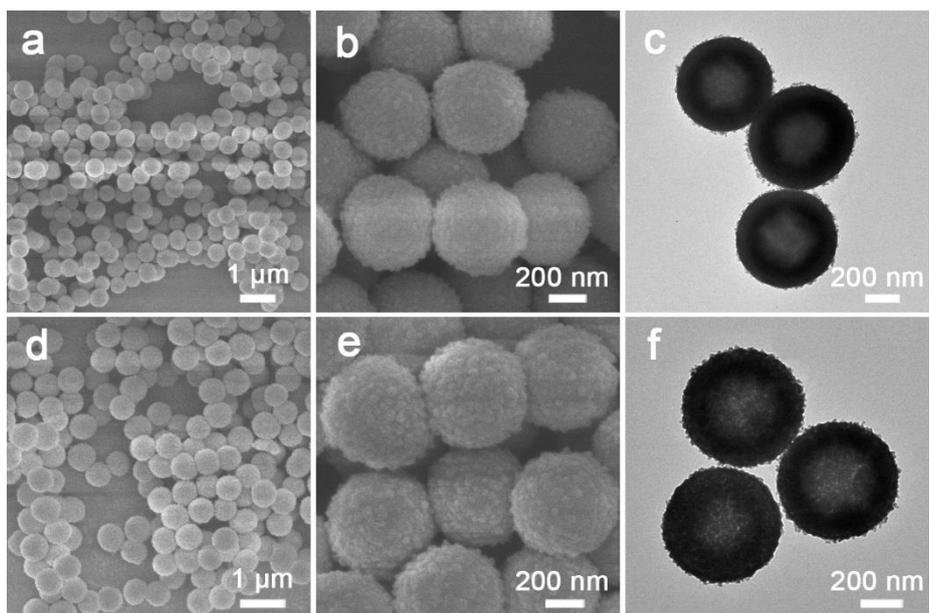
**Figure 3.** a,b,d,e) FESEM and c,f) TEM images of (a-c) Co-V precursor HSs, and (d-f)  $\text{Co}_3\text{V}_2\text{O}_8$  HSs.
