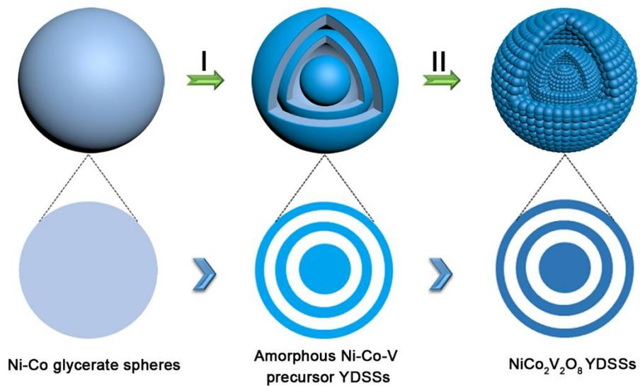
**Figure 1.** Schematic illustration for the synthesis of NiCo<sub>2</sub>V<sub>2</sub>O<sub>8</sub> YDSSs. Stage I: The formation of amorphous Ni-Co-V precursor YDSSs through an anion-exchange reaction; Stage II: Thermal treatment to generate NiCo<sub>2</sub>V<sub>2</sub>O<sub>8</sub> YDSSs.
