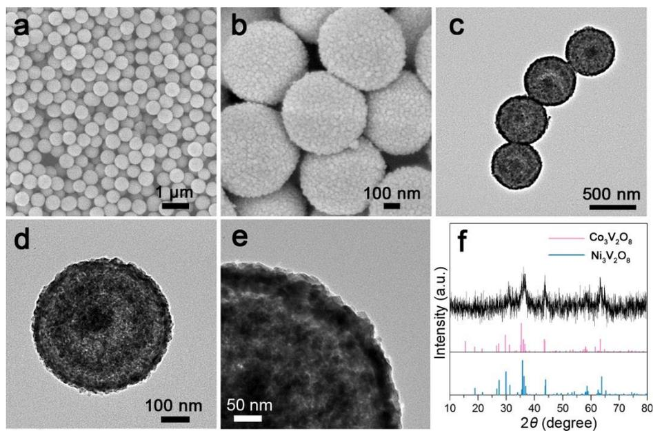
**Figure 2.** a,b) FESEM images, c-e) TEM images, and f) XRD pattern of the  $\text{NiCo}_2\text{V}_2\text{O}_8$  YDSSs.
