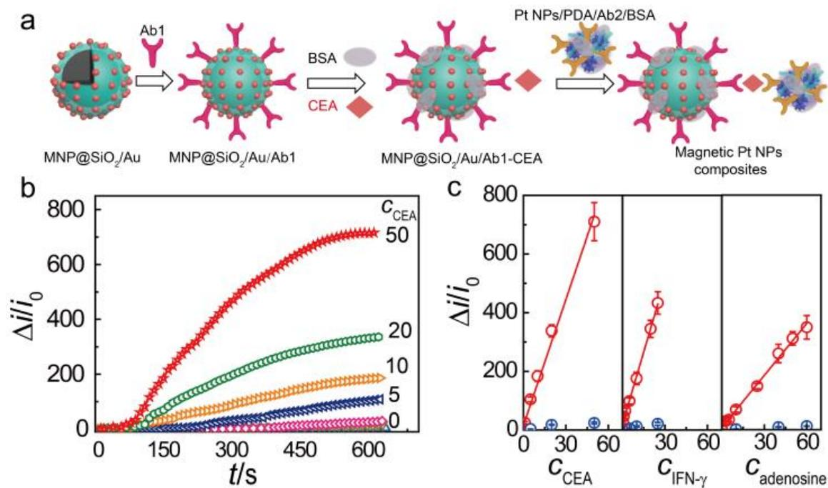
**Figure 3.** Sensing performance of tactile biosensors for various biomarkers. a) Schematic illustration of CEA immunoassay based on magnetic particles for separation and Pt NPs as labels. b) The current response of tactile biosensors for CEA with concentrations from 0 to 50 ng/mL. c) The linear detection of tactile biosensors for CEA (ng/mL), IFN- $\gamma$  (nM), and adenosine ( $\mu$ M), respectively.
