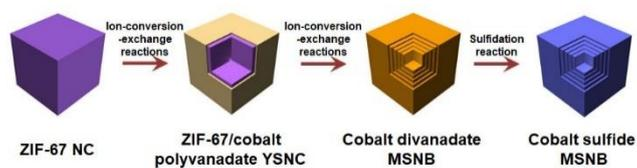
**Cobalt sulfide multi-shelled nanoboxes** are prepared through an ion-conversion-exchange strategy. With the structural and compositional advantages, these unique cobalt sulfide multi-shelled nanoboxes exhibit enhanced sodium storage performance when evaluated as anodes for sodium-ion batteries.
