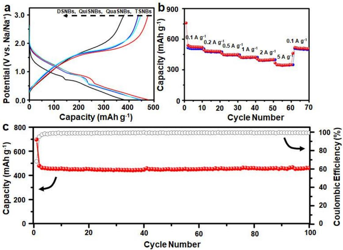
**Figure 5.** (a) The discharge-charge voltage profiles of cobalt sulfide MSNBs with different shell numbers for the second cycle at the current density of  $500 \text{ mA g}^{-1}$ . (b) The rate performance of cobalt sulfide TSNBs at various current densities and (c) cycling performance for 100 cycles at the current density of  $200 \text{ mA g}^{-1}$ .
