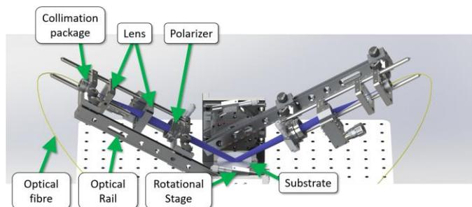
Fig. 1. Schematic model of the optical fiber interference lithography system (laser beam path is illustrated in blue).
