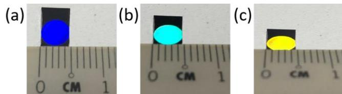
Fig. 4. Actual image of the samples showing different colors at a viewing angle of approximately (a) 10°, (b) 45° and, (c) 80°
