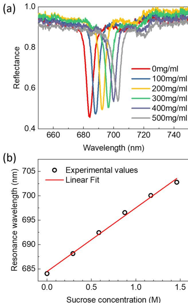
Fig. 6. (a) Spectrum of the reflected light collected by the spectrometer for each sucrose concentration. (b) plot of the observed resonance wavelength against the respective refractive index of the sucrose solutions
