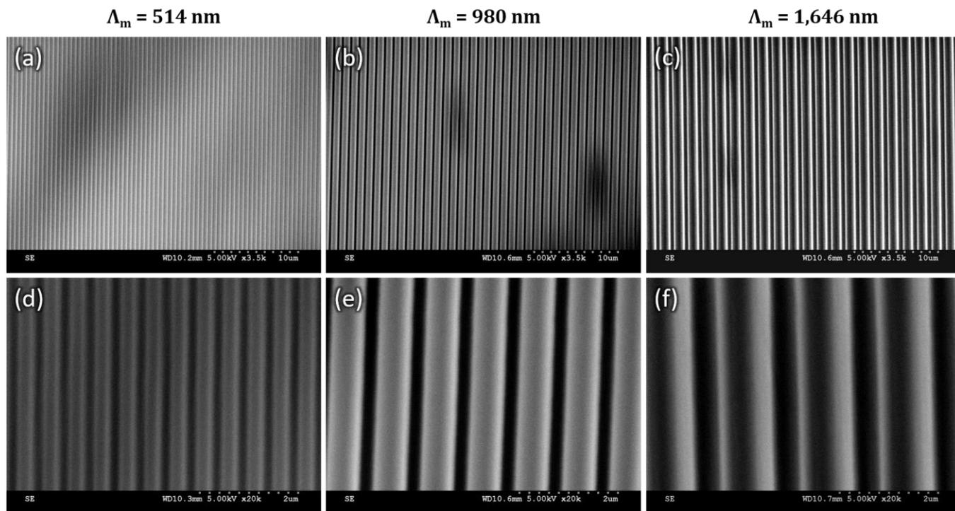
Fig. 2. SEM images of the respective grating features at (a)-(c) 3,500x and (d)-(f) 20,000x magnifications for the respective  $\Lambda_m$ .
