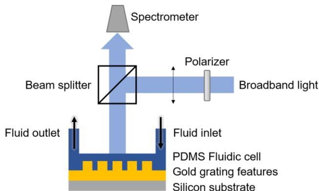
Fig. 5. Schematic illustration of the gold grating-coupled plasmonic biosensor configured for spectral interrogation mode.
