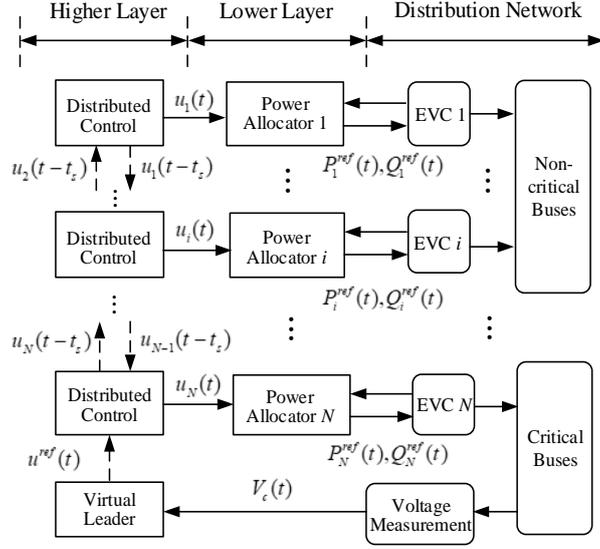
Figure 4: Configuration of the proposed voltage control scheme.
