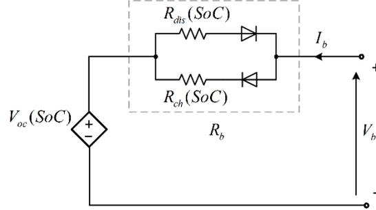
Figure 1: The equivalent circuit model of the lithium-ion battery.
