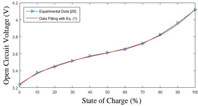
Figure 2: Comparison between data fitting result and experimental data in [28].
