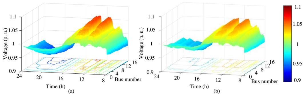
Figure 9: Voltage profiles of the distribution network in test case 2. (a) Uncoordinated EV charging. (b) Proposed voltage regulation method.
