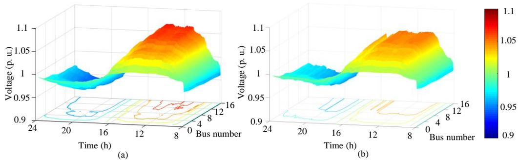
Figure 7: Voltage profiles of the distribution network in test case 1. (a) Uncoordinated EV charging. (b) Proposed voltage regulation method.
