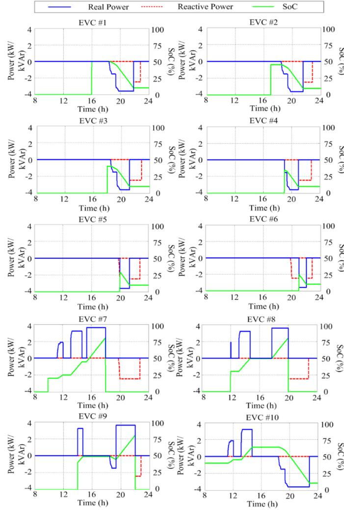
Figure 10. Real and reactive power outputs and SoC profile of each EVC.
