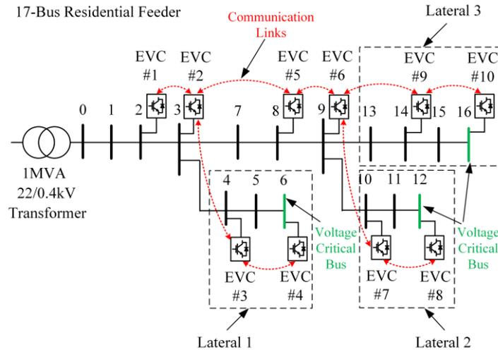
Figure 5: Configuration of the 17-bus residential distribution network.
