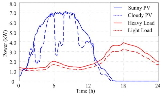
Figure 6: PV generation and load profiles for the simulation study.
