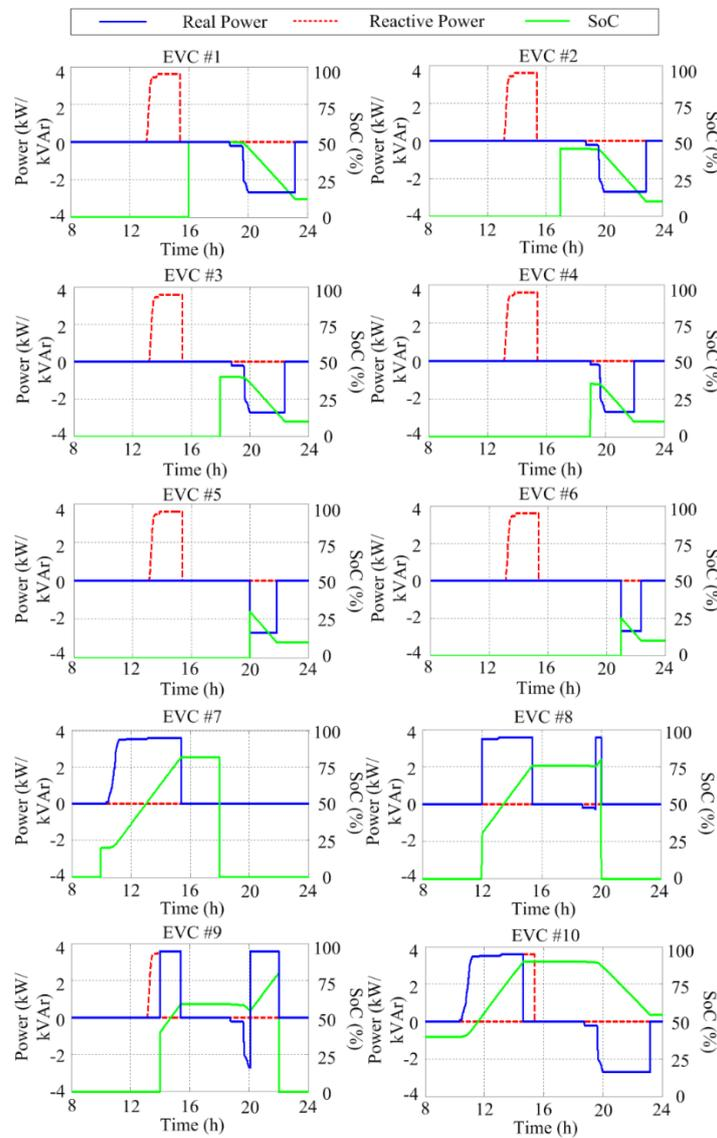
Figure 8: Real and reactive power outputs and SoC profile of each EVC.
