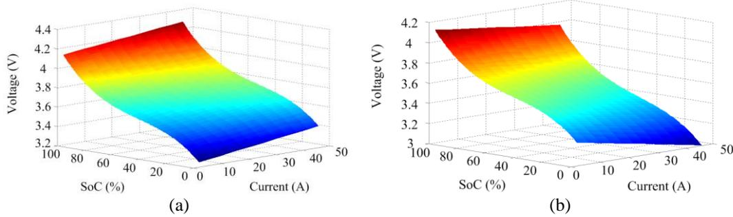
Figure 3: The charging/discharging characteristic of the lithium-ion battery. (a) charging process. (b) discharging process.
