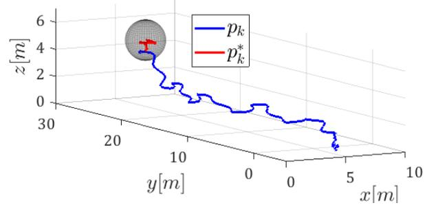
Fig. 6. Spatial trajectory of AUAV as measured by the anchor-based localization system. A ball of radius  $2$  m is cast around the last recorded position of TUAV to indicate when the AUAV reaches the target.
