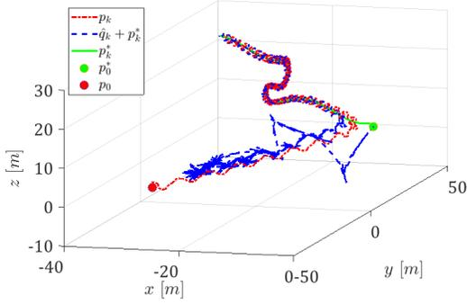
Fig. 2. 3-D visualization of the docking task with all possible corruptions against the ideal scenario. The initial position of the target is marked by the green circle and the UAV's initial position is marked by the red circle.
