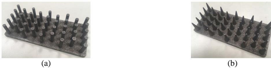
Fig. 3 Images of (a) cylindrical pin fin heat sink –  $C1$  and (b) parabolic pin fin heat sink –  $P1$ .
