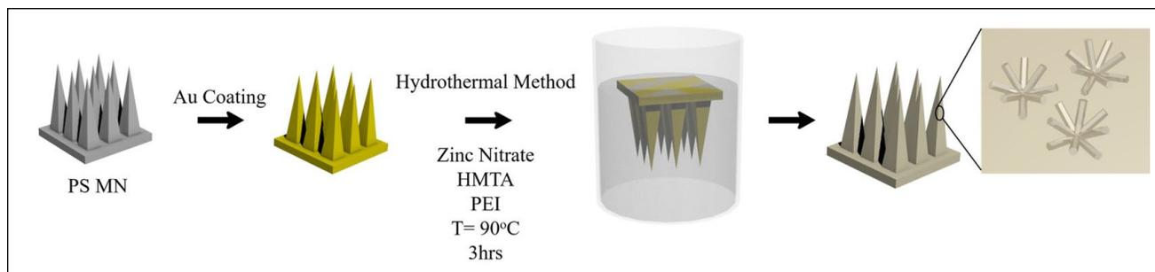
**Figure 1.** Schematic of ZnO nanobush generation on Au-coated PS MNs via hydrothermal growth method.
