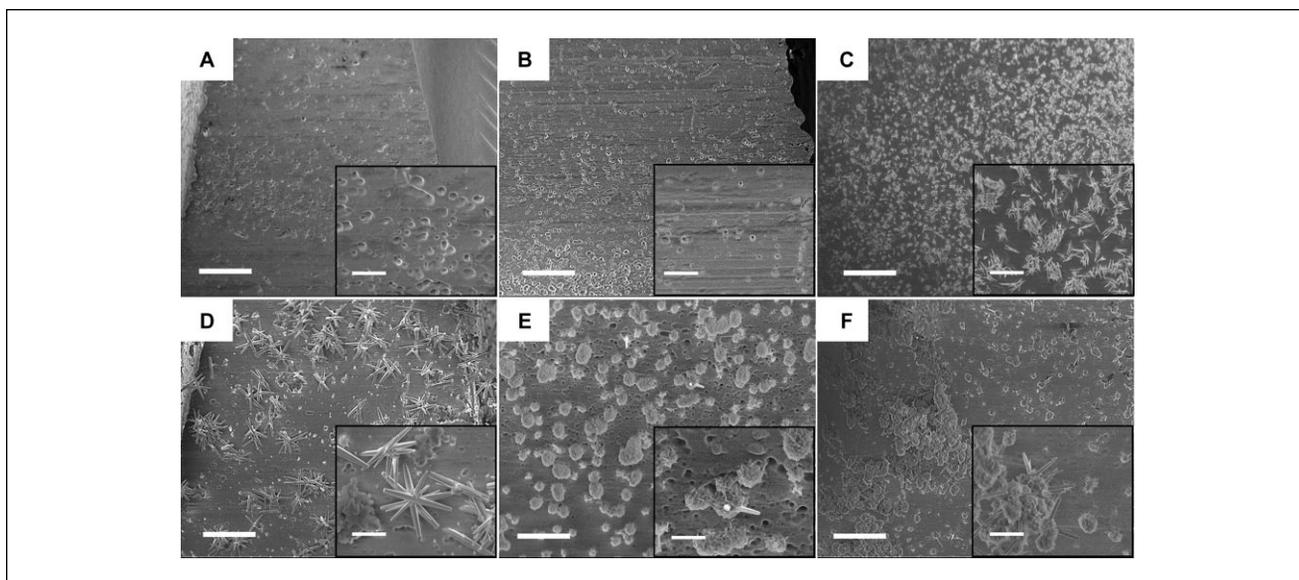
**Figure 3.** SEM images of ZnO nanobushes on Au-coated PS MN via the hydrothermal growth method with different precursor concentrations: (A) 10 mM, (B) 20 mM, (C) 30 mM, (D) 40 mM, (E) 50 mM, and (F) 60 mM. Insets show close-up views of the corresponding samples. Scale bars = 50  $\mu\text{m}$  and 5  $\mu\text{m}$  for the main images and insets, respectively.
