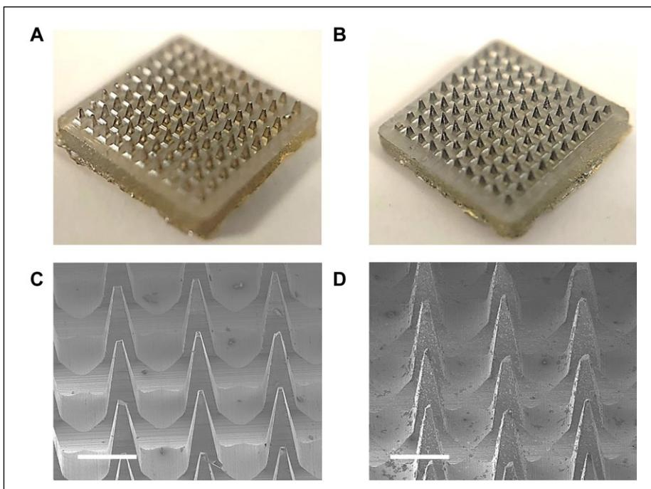
**Figure 2.** Optical images of (A) Au-coated PS MNs. (B) Au-coated PS MNs with ZnO nanobushes generated. (C) SEM images of Au-coated PS MNs. (D) Au-coated PS MNs with ZnO nanobushes generated. Scale bar = 500  $\mu\text{m}$ .
