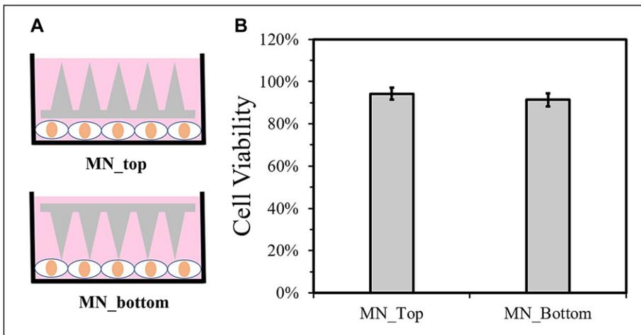
**Figure 5.** Cell viability test of NDFs with ZnO-coated PS MNs. (A) Schematic illustration of configuration of ZnO-coated PS MNs in the cell viability experiment. (B) Quantitative cell viability results of NDFs obtained from the AlamarBlue viability assay ( $n = 3$ ).
