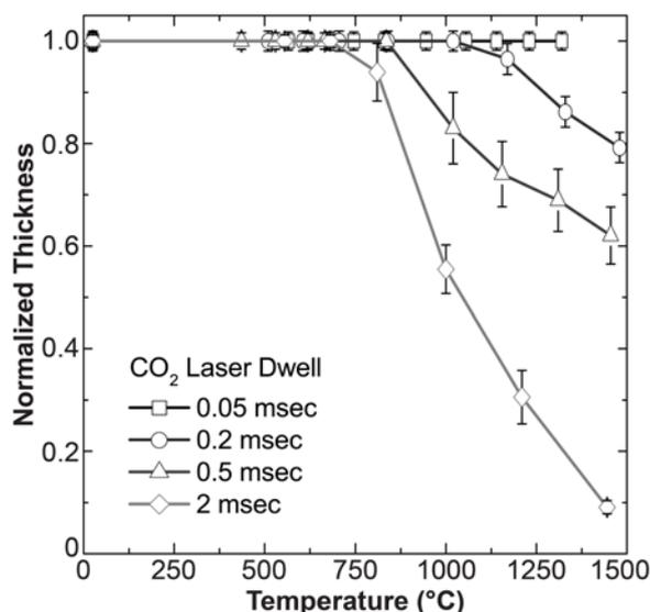
Figure 3. Film thickness plots of mesoporous resin template samples heated by a single laser irradiation for different submillisecond time dwells.<sup>34</sup>
