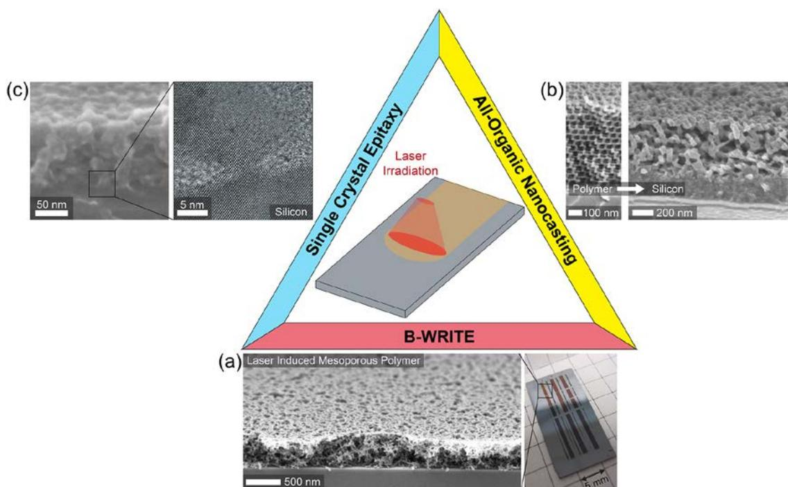
Figure 1. Transient laser heating-induced hierarchical structured materials. (a) Hierarchical mesoporous polymer nanostructures derived by B-WRITE.<sup>24</sup> (b) All-organic block copolymer templating of laser-induced 3D periodic silicon nanostructures.<sup>24</sup> (c) Excimer laser annealing of block copolymer templated single crystal epitaxial silicon nanostructures.<sup>23</sup>
