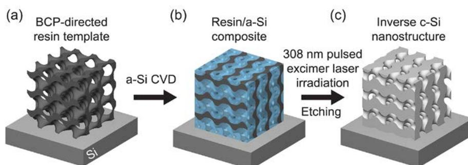
Figure 4. Schematic of complex block copolymer-directed single crystal silicon nanostructure formation by nanosecond pulsed excimer laser annealing.<sup>23,34</sup>
