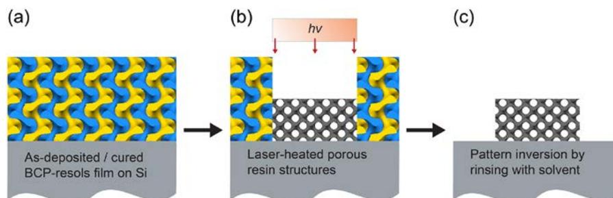
Figure 2. Schematic of block copolymer-induced writing by transient heating experiments (B-WRITE).<sup>24</sup>
