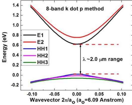
Fig. 2.  $\text{In}_{0.2}\text{Ga}_{0.8}\text{Sb}/\text{Al}_{0.2}\text{GaAsSb}$  QW bandgap calculation.
