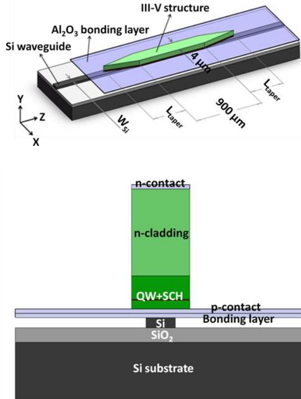
Fig. 1. Schematic diagram of the entire device and its cross section (not to scale).
