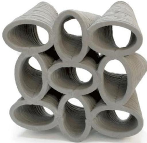
Figure 6. Concrete printed acoustic wall element (Valente et al. 2019).
