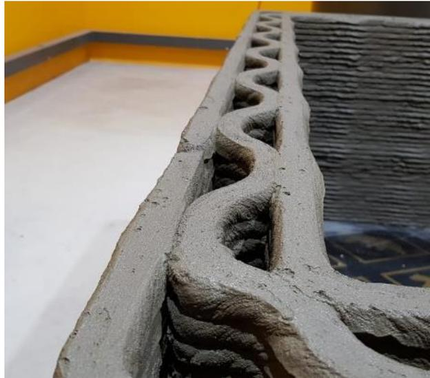
Figure 7. 3D printed lattice shape wall element printed in SC3DP, NTU.
