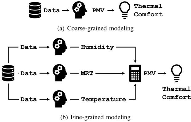
Fig. 1. System architectures of the coarse-grained and fine-grained thermal comfort modeling.
