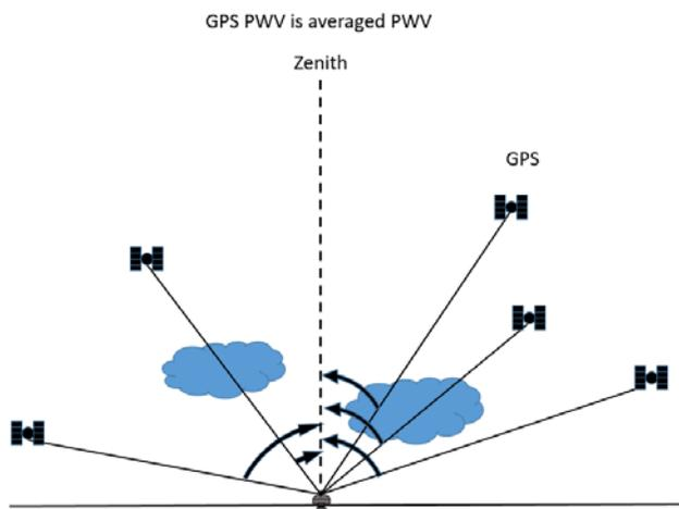
Fig. 4. Idea of zenith PWV determination.
