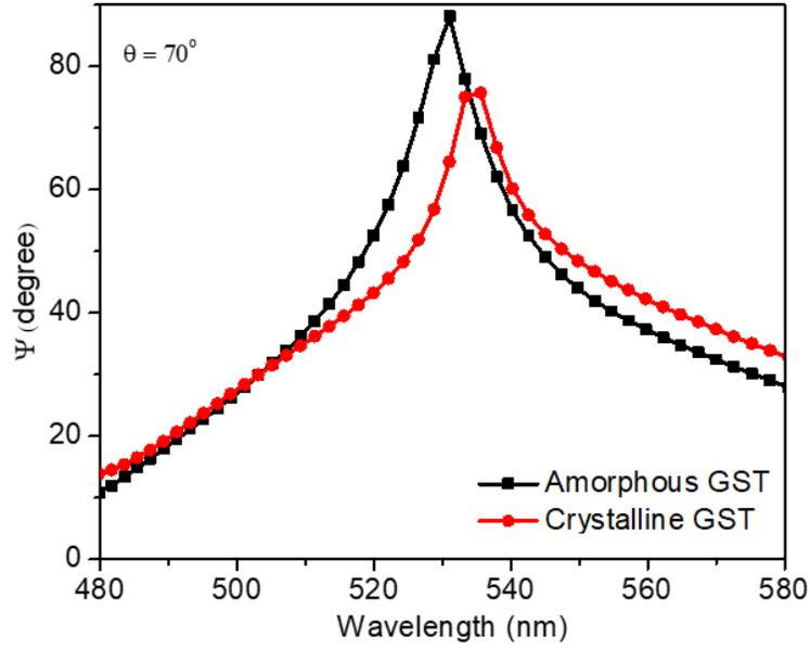
**Figure S8** Measured ellipsometry parameter,  $\psi$  of glass/GST/MMA at  $s$ -polarized Brewster angle ( $70^\circ$ ) for amorphous and crystalline phase of GST.
