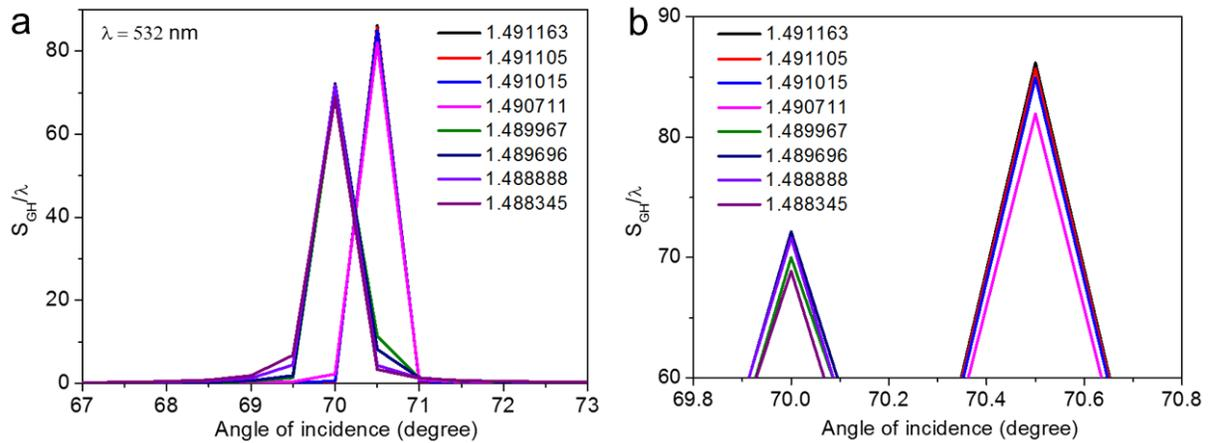
**Figure S3 (a)** Calculated tunable G-H shifts at 532 nm with change in refractive index of MMA. **(b)** Zoomed part of (a).
