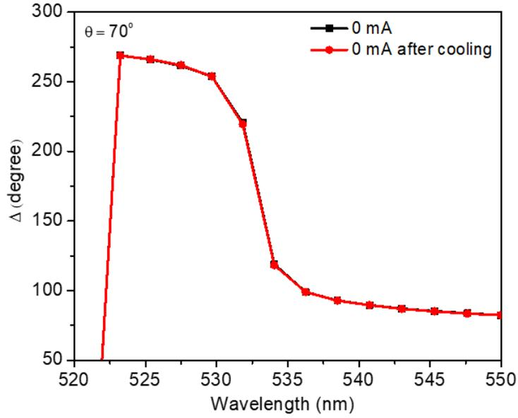
**Figure S6** Demonstration of reversible phase shift. Measured ellipsometry parameters,  $\Delta$  of Si/MMA stack in the forward and reverse direction at 0 mA (RT).
