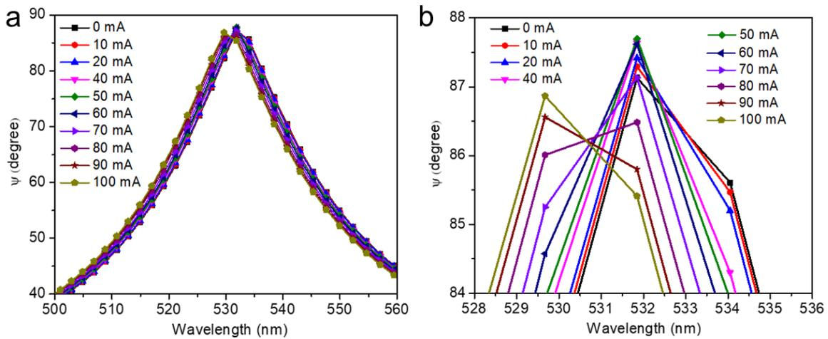
**Figure S5 (a)** Experimentally obtained ellipsometry parameter,  $\psi$  of Si/MMA stack at s-polarized Brewster angle ( $70^\circ$ ) with varying current. (b) Zoomed part of (a).
