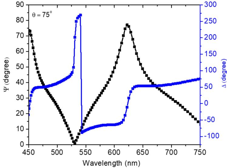
**Figure S10** Measured ellipsometry parameters,  $\psi$  and  $\Delta$  for glass/GST (amorphous)/MMA cavity at  $p$ -polarized Brewster angle of  $75^\circ$ .
