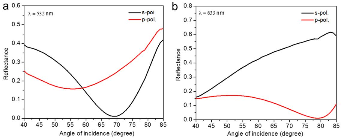
**Figure S7** Experimental demonstration of GBA in glass/GST (amorphous)/MMA stack. Angular reflectance spectrum for *s*- and *p*-polarizations (a) at 532 nm and (b) 633 nm.
