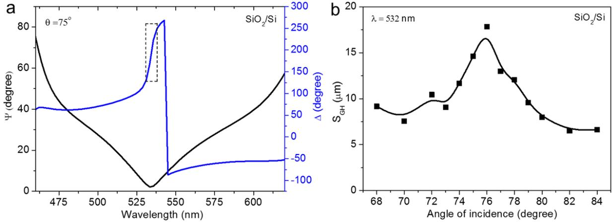
**Figure S2 (a)** Measured ellipsometry parameters of SiO<sub>2</sub>/Si stack at 75°, **(b)** Measured G-H shift as a function of incident angle at 532 nm.
