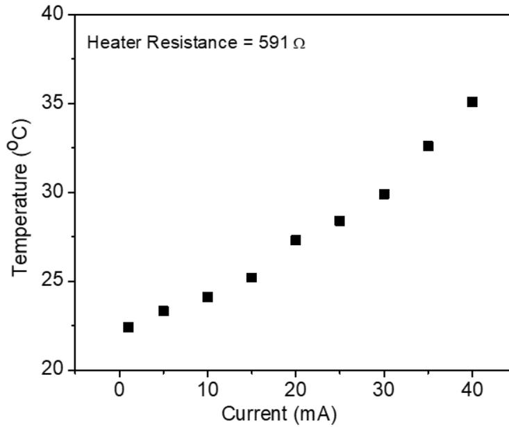
**Figure S9** Temperature calibration of microheater integrated glass/GST/MMA thin film absorber. Measured heater resistance at RT is  $591\Omega$ .
