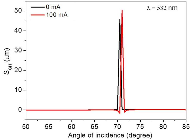
**Figure S4** Calculated G-H shifts of Si/MMA at 532 nm when applied current is 0 mA and 100 mA. A maximum thickness expansion of 3 nm and a slight surface roughness increase of 0.25 nm are obtained when the current is increased from 0 to 100 mA. Here, we compare the simulated G-H shifts obtained at 532 nm for 0 mA and 100 mA (with expanded thickness and change in refractive index of MMA layer) and found that G-H shifts considerably vary near the Brewster angle.
