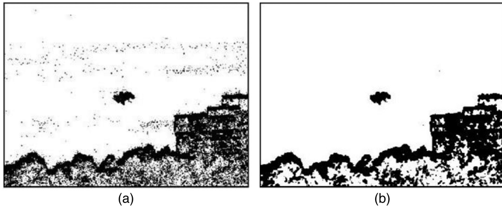
Fig. 3 Event-based frames in drone surveillance tasks. (a) Without denoising operation. (b) With denoising operation.
