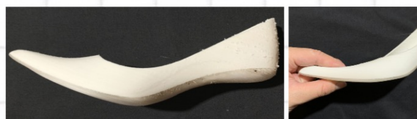
Figure 7: Flexible upper (TPE) & hard sole (PC) printed with the Arburg Freeformer.
