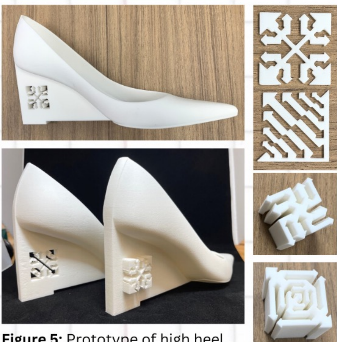
Figure 5: Prototype of high heel and patterns printed with the SLS printer in TPU.
