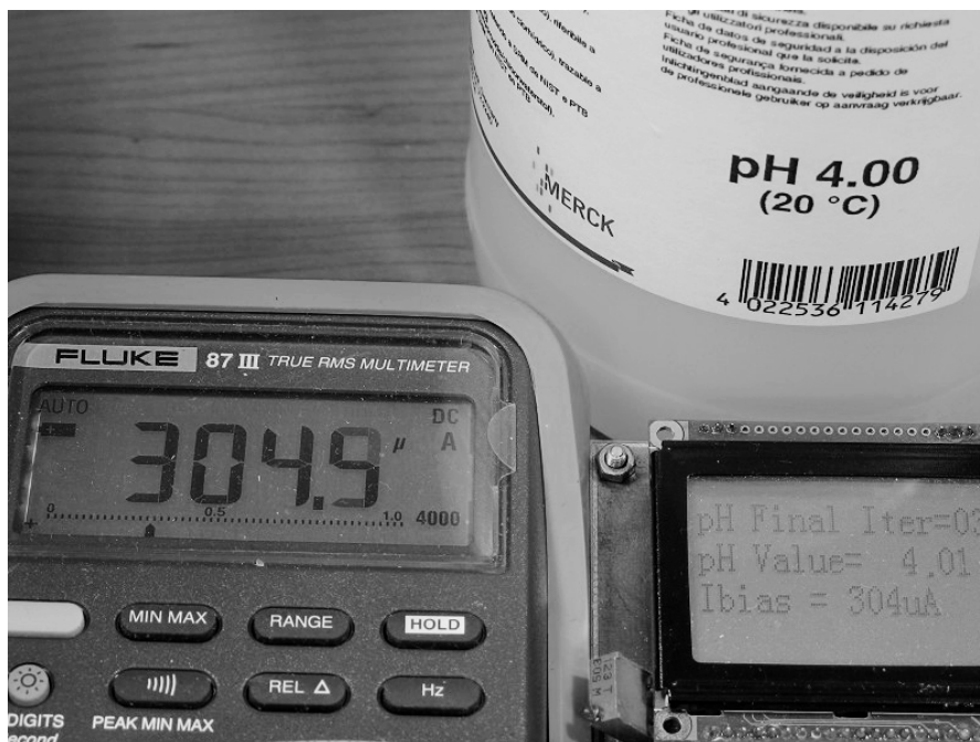
Fig. 7.14 LCD display of measurement result of optimum biasing current and pH value in pH4 buffer solution at 50°C
