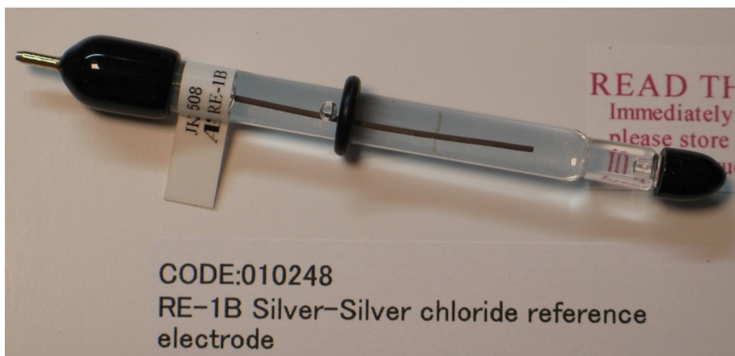
Fig. C.1 Photo of Ag/AgCl Reference Electrode
