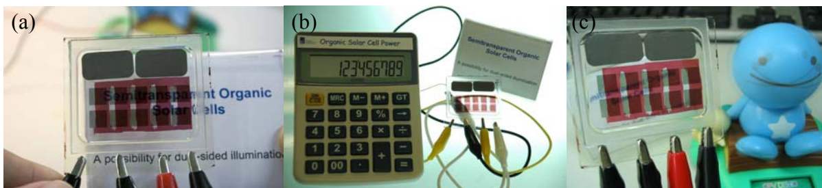
Figure 5.8: (a) A lateral integrated translucent PSC demonstrator with total active area of 1.5\text{cm}^2 . (b) a photo picture of a calculator which was powered up using a translucent PSC, and (c) a photo picture of electronic device (toy) running using the power generated by a translucent PSC.
