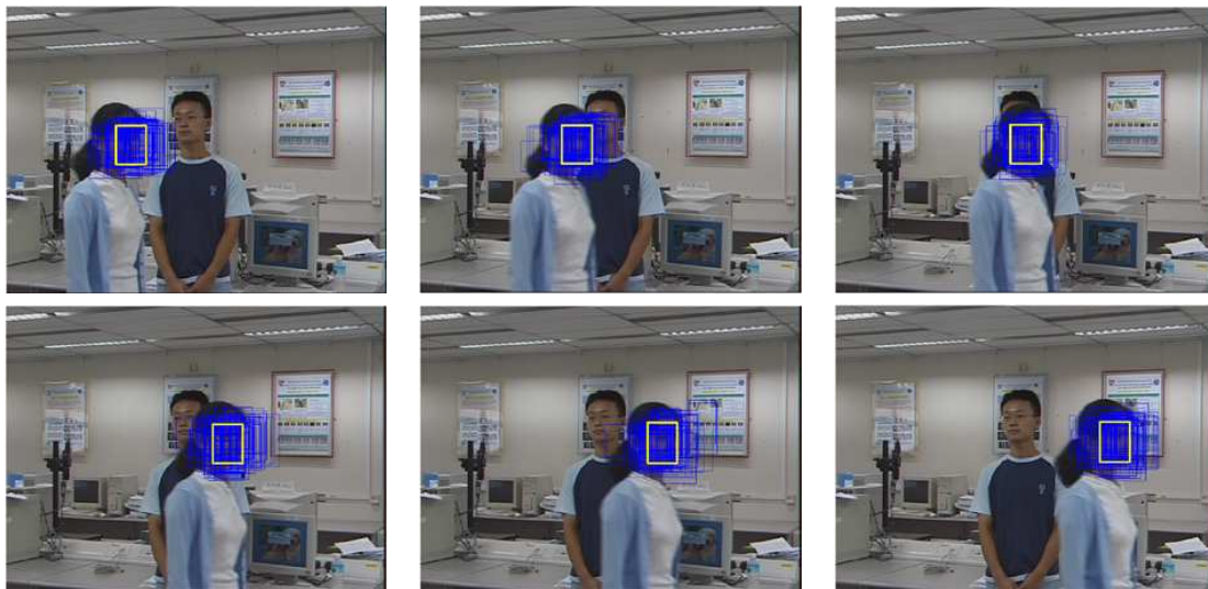
Figure 3.3: Face tracking in clutter sequence. Frames 4, 6, 8, 10, 11 and 13 are shown. The LEPF approach is able to track the identified face despite color clutter. It has the ability to keep track momentarily multiple modes and predict over time. So when the target moves out of the clutter, the tracker can still keep track of the target.
