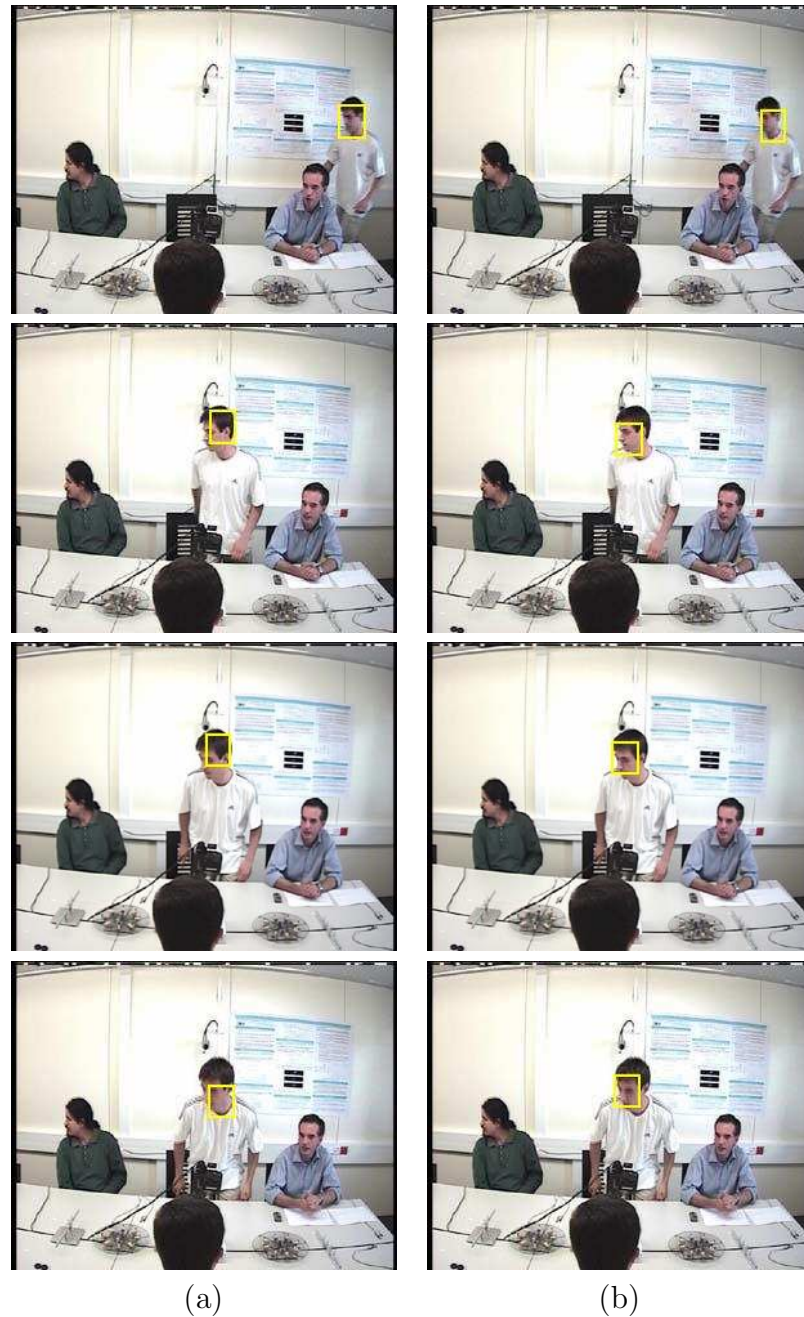
Figure 4.4: Comparison of experimental results on face tracking in the frame 3, 60, 65 and 70, the left column shows the results of particle filter algorithm and the right column shows the results of transductive particle filter algorithm.
