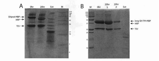
**Figure 3-10.** TEV cleaving and purification of SHprot (A) and long-SH-TM (B) with organic solvent extraction. TEV and fusion proteins were mixed together for cleaving reaction (0hr) with gentle shaking for 20hr at room temperature. The proteins were precipitated with TCA and lyophilized. The proteins were extracted with methanol and the supernatant was collected by centrifugation at 12,000 g (Ext).
