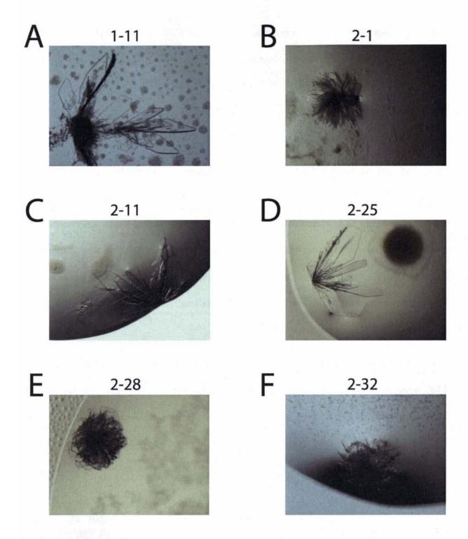
Figure 3-32. Crystal formed by SH-TM reconstituted into β-OG using the MemGold sparse matrix screening kit. Plates like crystals are found in condition 1-11 (A), 2-11 (C), and 2-25 (D). Small cluster of plates like crystals are found in condition 2-1 (B), 2-28 (E), and 2-32 (F).
