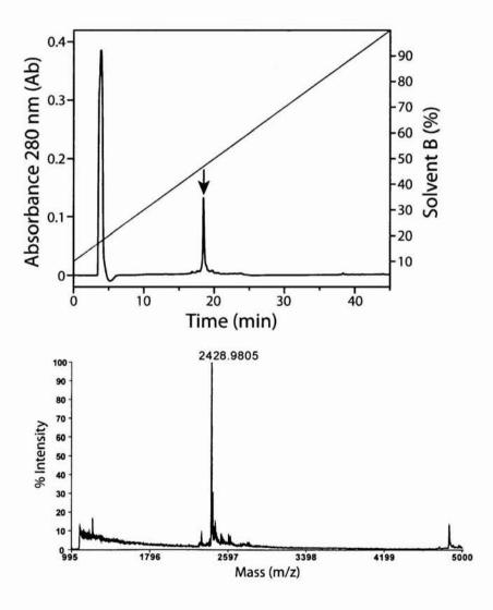
Figure 3-4. RP-HPLC purification of SH-C20. A C18 RP-HPLC chromatography column was used to purify SH-C20 using linear acetonitrile gradient, monitored at 220nm. The peak
