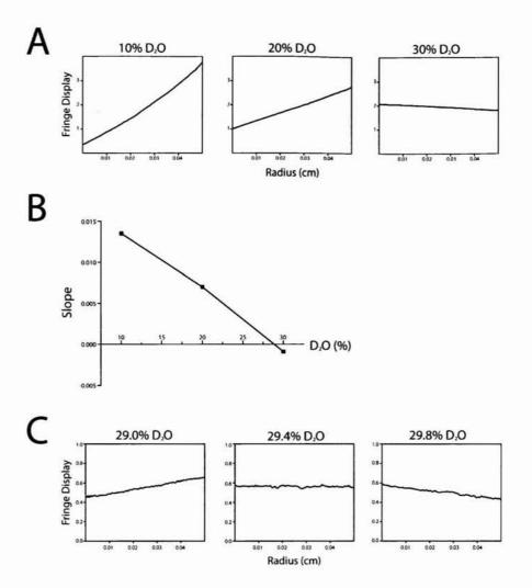
Figure 3-17. Density matching of 5 mM C14SB with  $D_2O$  in buffer containing 50 mM Tris-HCl, and 100 mM NaCl, pH 7.3. (A) Interference scans of various concentration of  $D_2O$ . (B) The plot of slope of micelle distribution as a function of  $D_2O$  percentage. (C) Final density matching for 5 mM C14SB based on the plot at (B).
