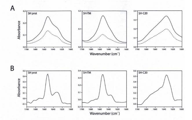
**Figure 3-28.** ATR-FTIR spectra and Fourier self deconvolution of SHprot, SH-TM and SH-C20 reconstituted in DMPC bilayers supported on germanium plate in D<sub>2</sub>O. (A) Polarized ATR-FTIR of SHprot, SH-TM and SH-C20 obtained at parallel (solid line) or perpendicular (dotted line) polarized light. (B) Fourier self deconvolution of these samples obtained with a bandwitdth of 20 cm<sup>-1</sup> and an enhancement factor of 2.0.
