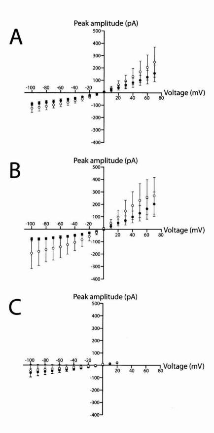
**Figure 3-38.** Whole-cell current-voltage plot of SH protein (A), H22A mutant (B), and vector alone-transfected HEK293 cells (C) at neutral (pH 7.2) (closed circle), and acidic (pH.5.5) (opened circle) solution. The cells were held at 0 mV and stepped to various potentials from 100 to 70 mV (in steps of 10 mV). Three independent data sets were used to plot the curve.
