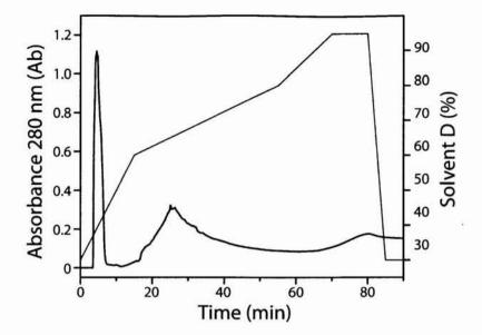
**Figure 3-2.** RP-HPLC purification of full-legth SH protein. A C4 RP-HPLC chromatography column was used to purify SHprot from major contaminants on the basis of hydrophobicity using linear isopropanol gradient, monitored at 220nm.
