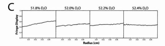
**Figure 3-16.** Density matching of 10 mM DPC with  $D_2O$  in buffer containing 50 mM Tris-HCl, and 100 mM NaCl, pH 7.3. (A) Interference scans of various concentration of  $D_2O$ . (B) The plot of slope of micelle distribution as a function of  $D_2O$  percentage. (C) Final density matching of 10 mM DPC based on the plot at (B).
