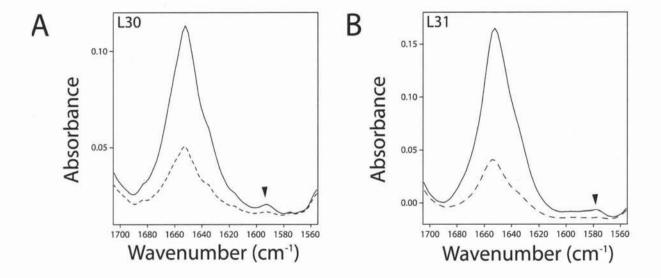
Figure 3-34. Polarized ATR-FTIR absorbance spectra of SH-TM reconstituted in DMPC bilayers in the amide I region of L30 (A) and L31 (B). The position of the labeled C=O stretching band is indicated with an arrow. Solid line and broken line indicate spectra obtained at parallel or perpendicular polarization, respectively.
