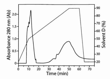
**Figure 3-5.** RP-HPLC purification of SH44 thioester. A C4 RP-HPLC chromatography column was used to purify SH44 thioester from major contaminants on the basis of hydrophobicity using linear isopropanol gradient, monitored at 220nm.
