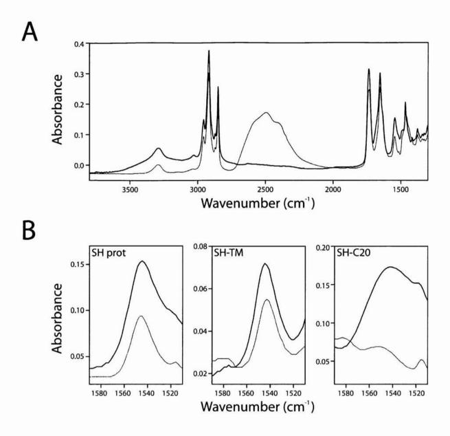
Figure 3-30. Hydrogen-deuterium exchange of SHprot, SH-TM, and SH-C20 reconstituted in supported DMPC bilayers. Dark and grey lines correspond to spectra recorded in  $H_2O$  and  $D_2O$ , respectively. (A) Overview of SHprot hydrogen-deuterium exchange, the spectra recorded in  $D_2O$  has a broad band centered at 2500 cm-1. (B) Amide II band of SHprot, SH-TM, and SH-C20 in  $H_2O$  and after I hour exposure to  $D_2O$ .
