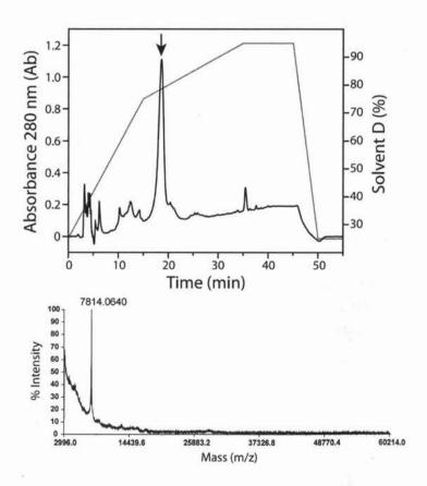
**Figure 3-11.** RP-HPLC purification of SHprot. A C4 RP-HPLC chromatography column was used to purify SHprot from major contaminants on the basis of hydrophobicity using linear isopropanol gradient, monitored at 220nm. The peak corresponding to purified SHprot is indicated by an arrow and the mass spectra analysis is shown at the lower panel.
