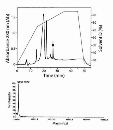
**Figure 3-12.** RP-HPLC purification of long SH-TM. A C4 RP-HPLC chromatography column was used to purify long SH-TM from major contaminants on the basis of hydrophobicity using linear isopropanol gradient, monitored at 220nm. The peak corresponding to purified long SH-TM is indicated by an arrow and the mass spectra analysis is shown at the lower panel.
