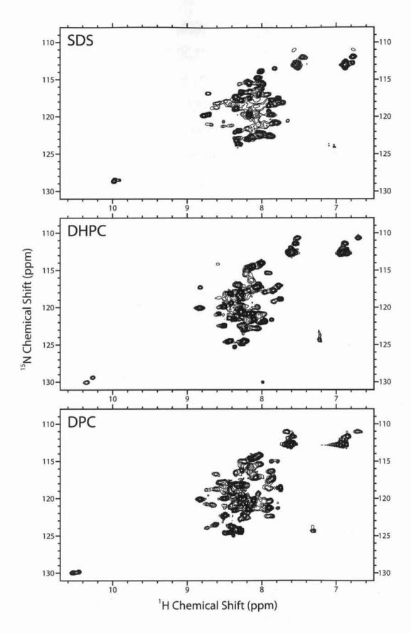
**Figure 3-31.** The effect of different micellar environments on SH protein illustrated with  $^{1}\text{H}/^{15}\text{N-HSQC}$  spectra. The detergents SDS (Top), DHPC (Middle), and DPC (Bottom) were used to obtain the spectra.
