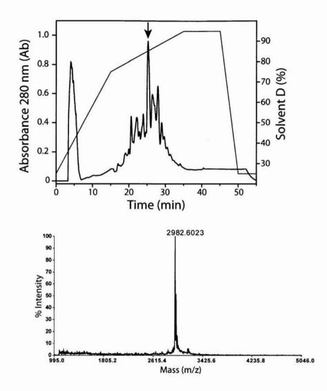
**Figure 3-1.** RP-HPLC purification of SH-TM. A C18 RP-HPLC chromatography column was used to purify SH-TM using linear isopropanol gradient, monitored at 220nm. The peak corresponding to purified SH-TM is indicated by an arrow and the mass spectra analysis is shown at the lower panel.
