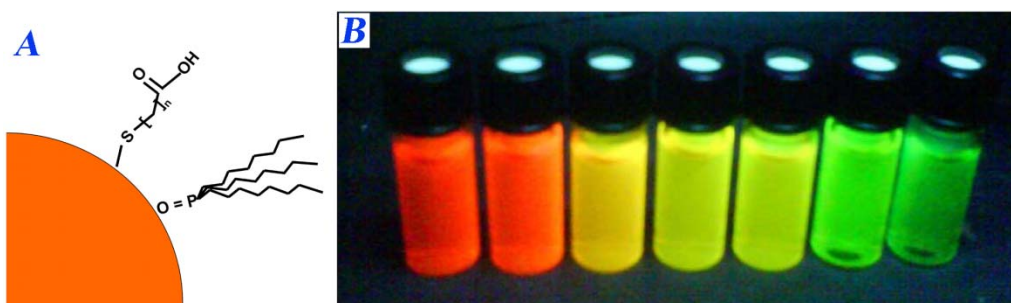
Figure 2.1 (A) Scheme of the core and coating of QDs. (B) A series fluorescence of MSA–CdTe QDs of different sizes under UV irradiation.
