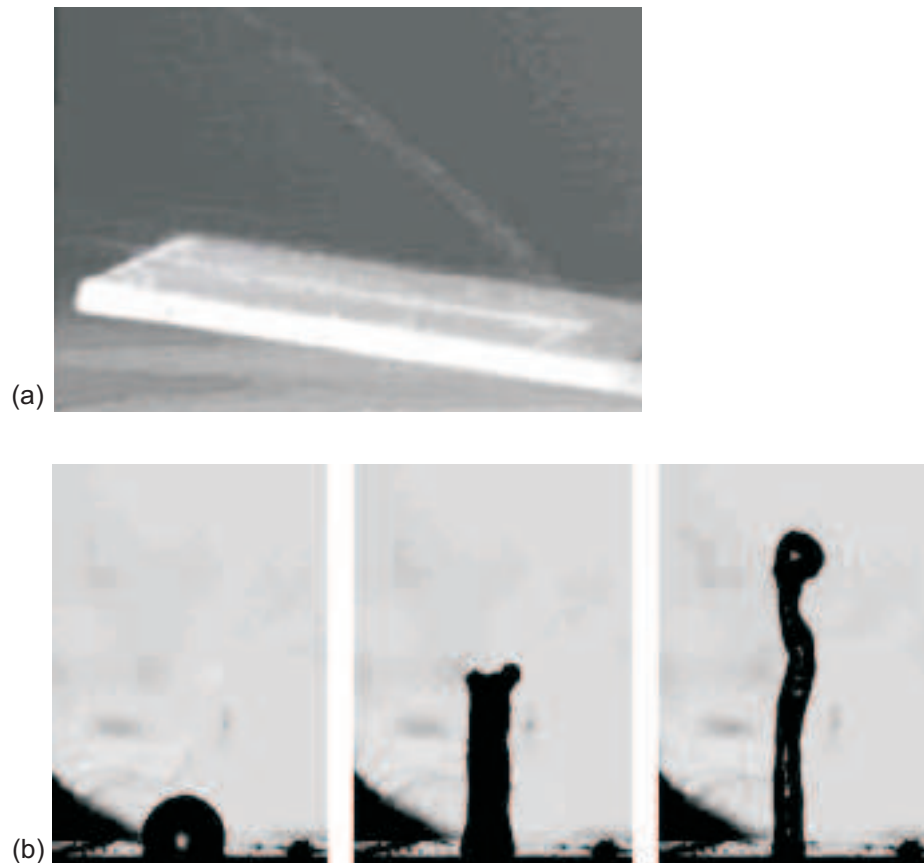
Figure 2.9: (a) Droplet jetting induced by a single SAW; (b) Snapshots of a droplet jetting induced by a pair of SAWs.
