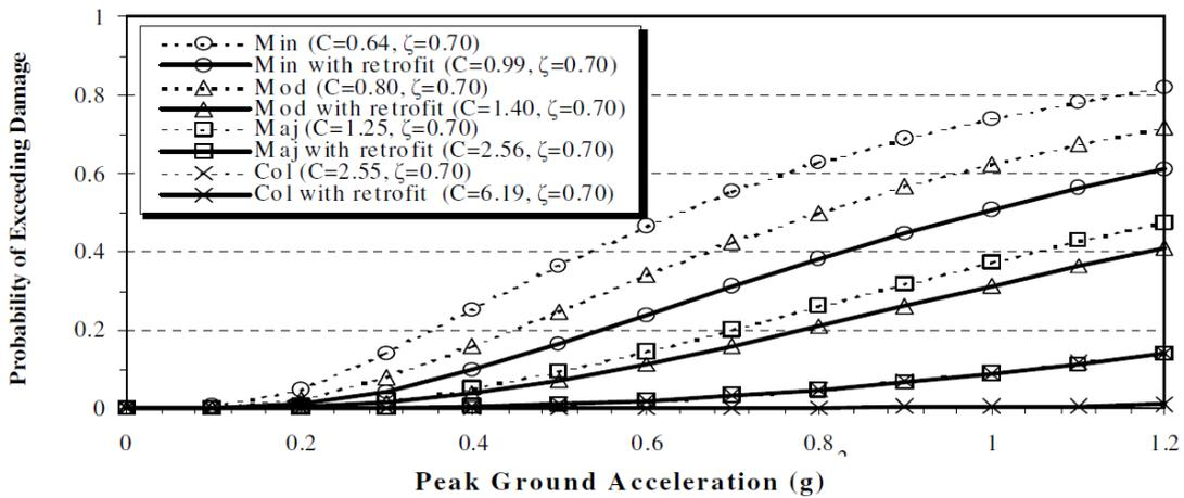
**Figure 7.6 Fragility Curve for Bridges With and Without Retrofit**
