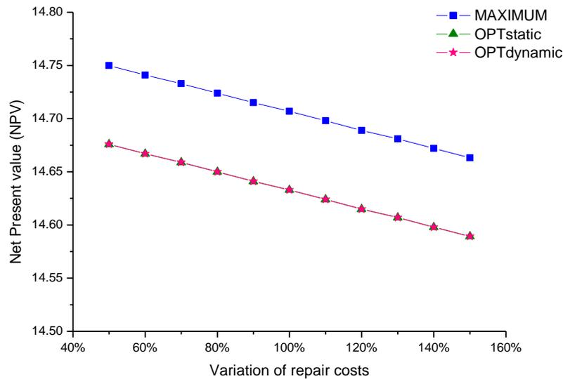
**Figure 6.14 NPVs for Different Repair Costs**
