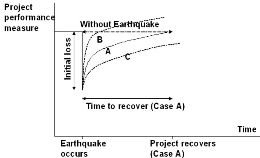
**Figure 7.4 Schematic of Catastrophe Recovery**
