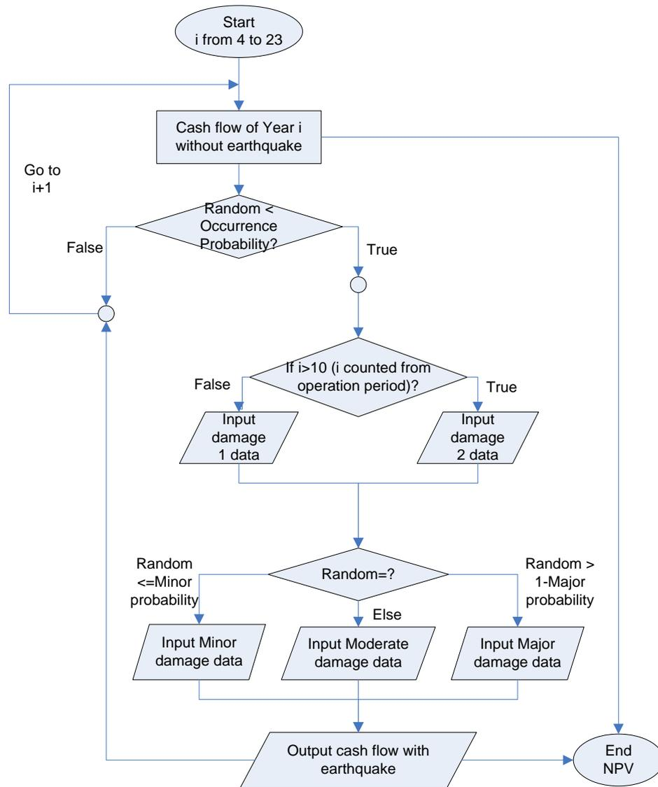
**Figure 7.7 Flow Chart of the Programming of Seismic Impact on Cash Flow Model**
