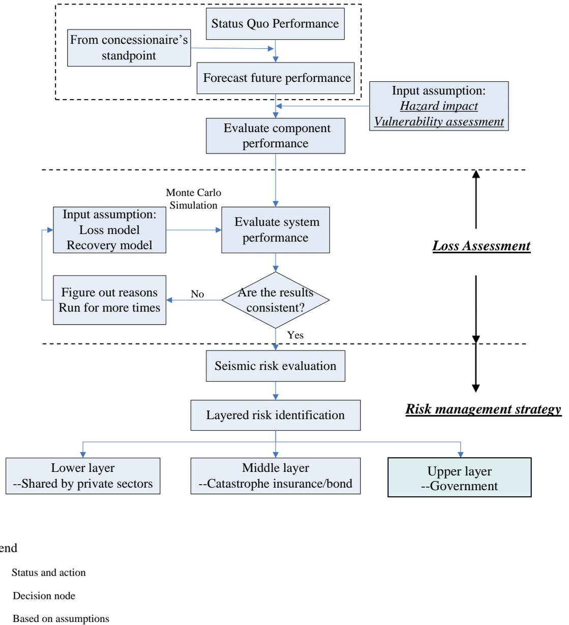
**Figure 7.1 Framework of Seismic Risk Analysis for A Highway Project**
