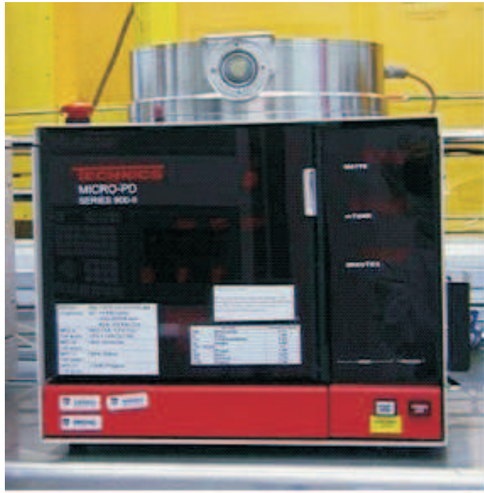
Figure 6.7 RIE machine used for oxygen plasma etching.
