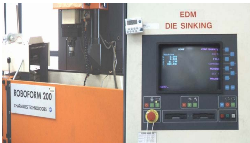
Figure 3-3 CHARMILLES ROBOFORM 200 EDM Machine
