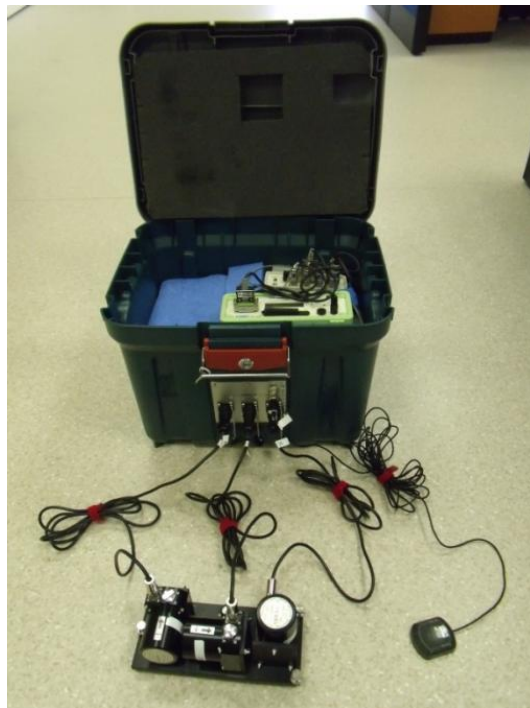
Figure 2-3 A set of tri-axial velocity seismometer
