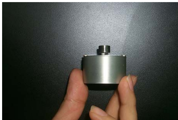
Fig. 2.8 Portable shaker for characterizing mechanical property of human skin
