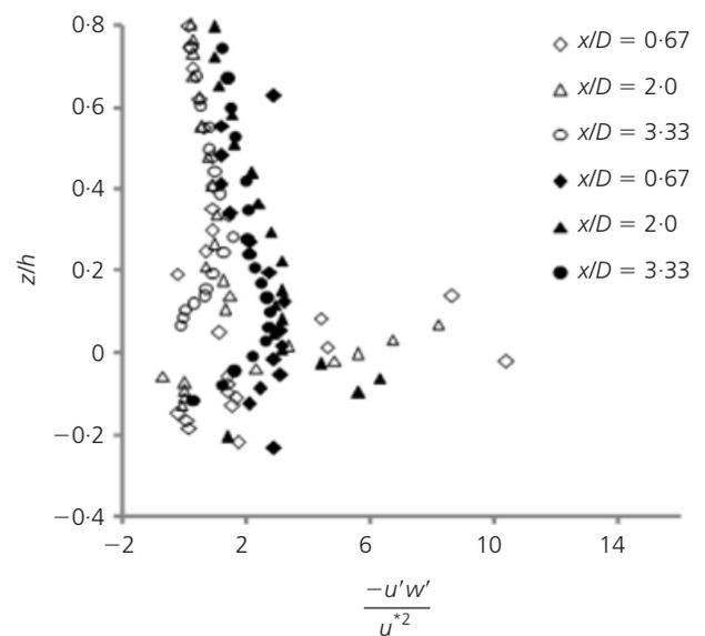
Figure 7. Normalised Reynolds stress profiles in the upstream plane of the cylinder (solid symbols, no jet and suction; open symbols, with jet and suction)
