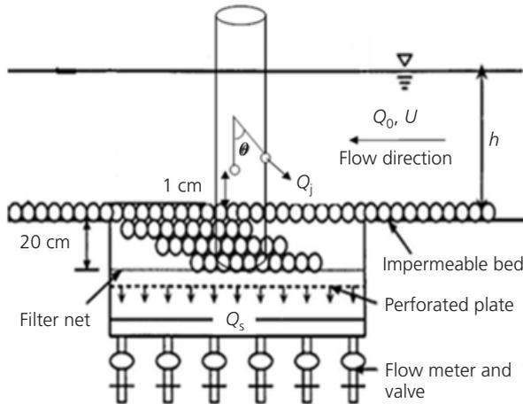
Figure 1. Layout of the seepage zone
