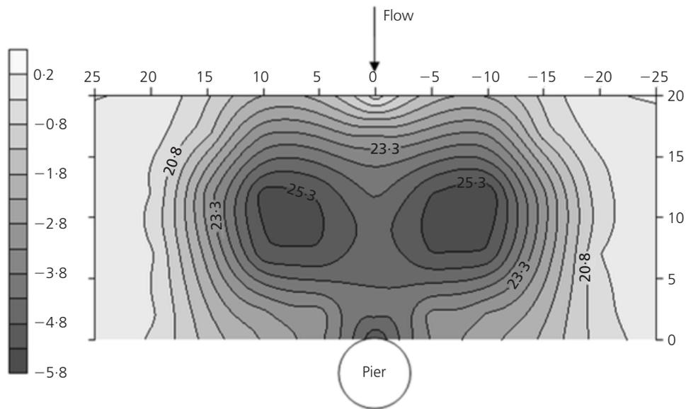
Figure 3. Equilibrium scour hole profile for bed suction and 3-jet injection with  $h = 10.5$  cm for  $\theta = 45^\circ$  (test B2) (units in cm)
