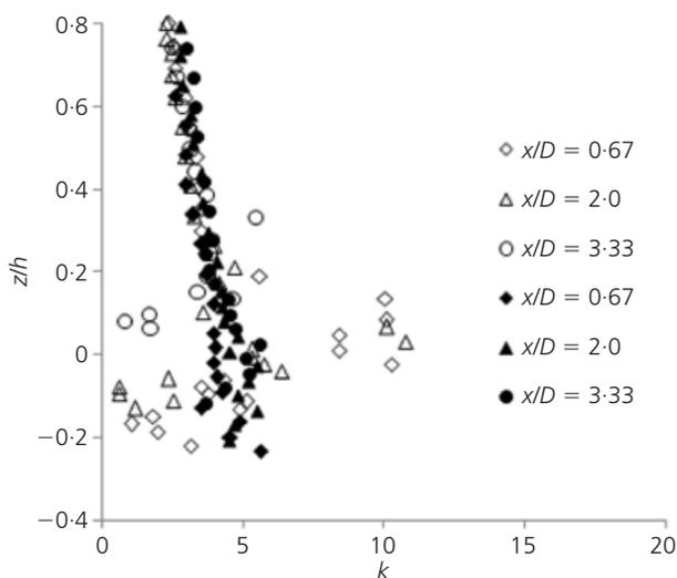
Figure 8. Turbulent kinetic energy in the upstream plane of the cylinder (solid symbols, no jet and suction; open symbols, with jet and suction)
