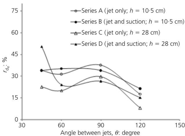
Figure 6. Effect of jet angle,  $\theta$ , on  $r_{de}$  with three jet outlets ( $Q_j = 0.015$  l/s)
