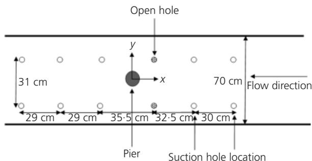
Figure 2. Plan view of the seepage zone
