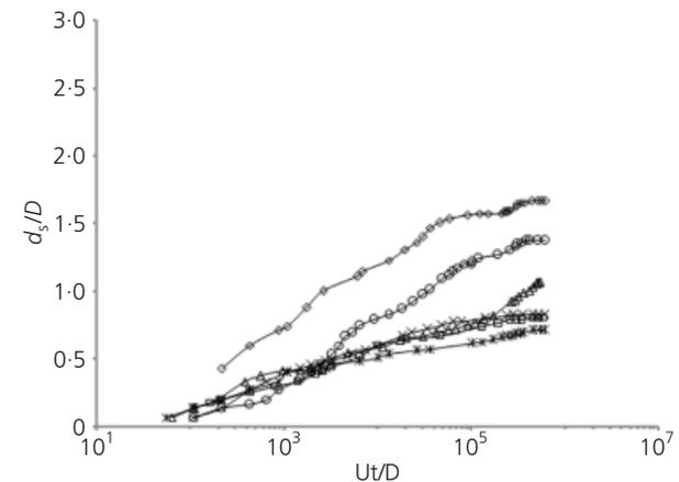
Figure 5. Dimensionless time evolution of the scour depth in front of the pier for water depths 28 cm (series D) and 10.5 cm (series B)
