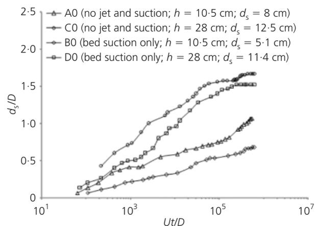
Figure 4. Dimensionless time evolution of the scour depth in front of the piers for water depths 10.5 and 28 cm
